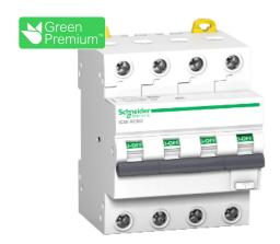
Residual current breaker with overcurrent protection (RCBO), Acti9 iC60, 4P, 10A, C curve, 6000A/6kA, A type, 30mA
