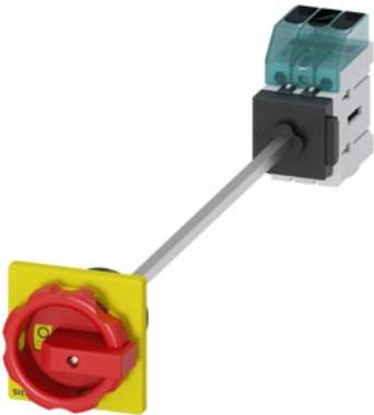
Load disconnector 3LD3, I<sub>u</sub> 40 A Main switch 3-pole Rated operating capacity at AC-23 A at 400 V 18.5 kW floor mounting Basic switch with door coupling Central hole mounting 22.5mm Rotary actuator red / yellow 66 x 66 mm
