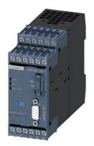
Basic unit SIMOCODE pro V MR, MODBUS RTU interface 57.6 Kbps, RS 485, 4I/3O freely parameterizable, Us: 110...240 V AC/DC, input for thermistor connection Monostable relay outputs, expandable by extension modules
