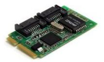
The MPEXSATA22I 2-Port Mini PCIe to SATA Controller Card lets you add 2 SATA 3Gbps connectors to a small form factor or embedded system, through a Mini PCI Express (Mini Card) expansion slot.
