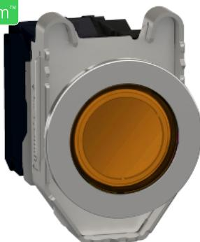
**Illuminated push button, Harmony XB4, metal, orange flush mounted, 30mm, universal LED, plain lens, 1NO + 1NC, 24V AC DC**
