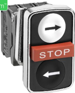
Triple headed push button, Harmony XB4, white flush, red projecting, black flush pushbutton, 22mm, spring return, 1NO + 1NC
