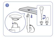
Insert the stand neck into the stand base in the direction shown in the figure. Tightly fasten the connecting screw at the bottom of the stand base.
