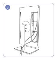
Connect the cables to their correct ports, and then arrange each of the two cables through either side of the COVER-STAND CABLE, as shown in the figure.
