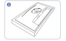
Place the protective Styrofoam (cushion) included in the package on the floor and place the product facing down on the Styrofoam, as shown in the image.
