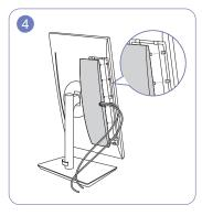
Arrange the cables through the groove on the COVER-REAR, and then attach the COVER-REAR SUB. When you attach the COVER-REAR SUB, please aim six ribs of the COVER-REAR SUB to the bottom holes of the COVER-REAR at first.
