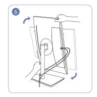
Rotate the machine to the horizontal position.
