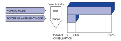
**NOTE** Even when using the power management mode, the monitor consumes electricity. Turn off the Power Switch whenever the monitor is not in use, during the night and weekends, to avoid unnecessary power consumption.
