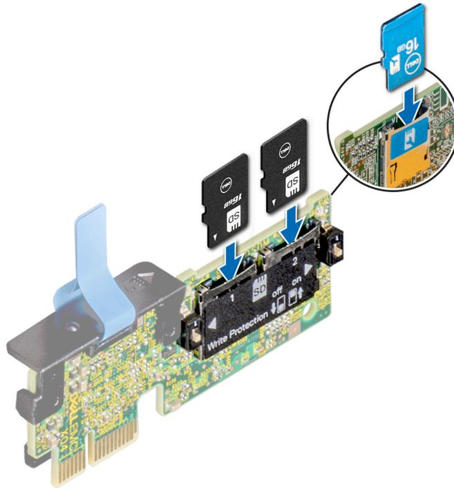
Figure 78. Installing the MicroSD card
