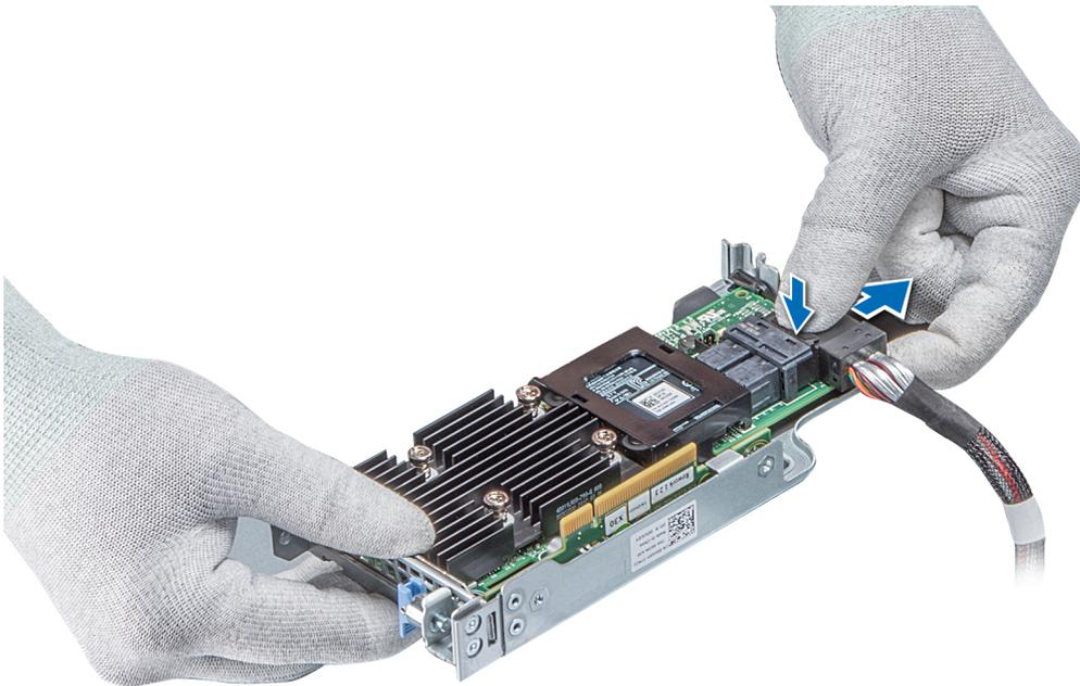
**Figure 70. Disconnecting the cable from internal PERC card**
