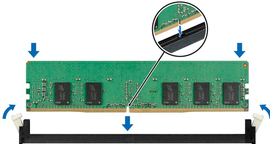
**Figure 42. Installing a memory module**
