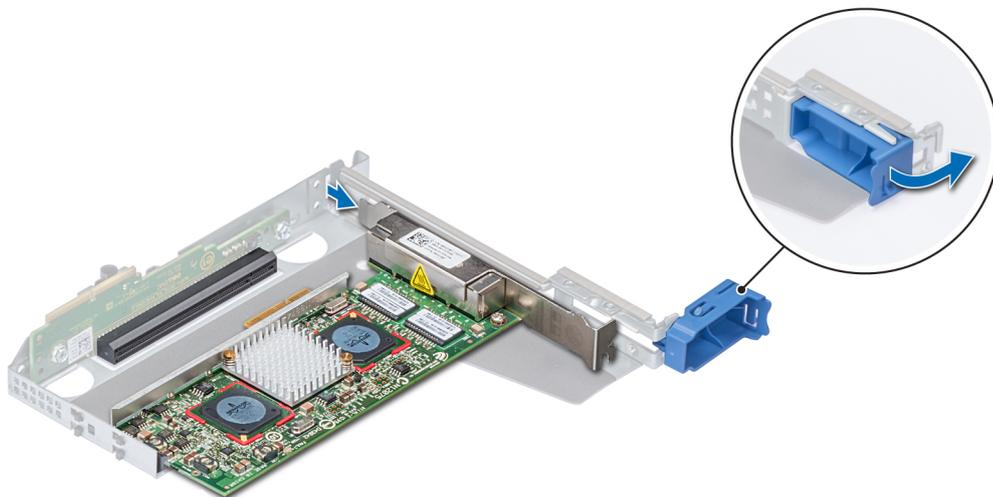
Figure 62. Removing expansion card from riser 1
