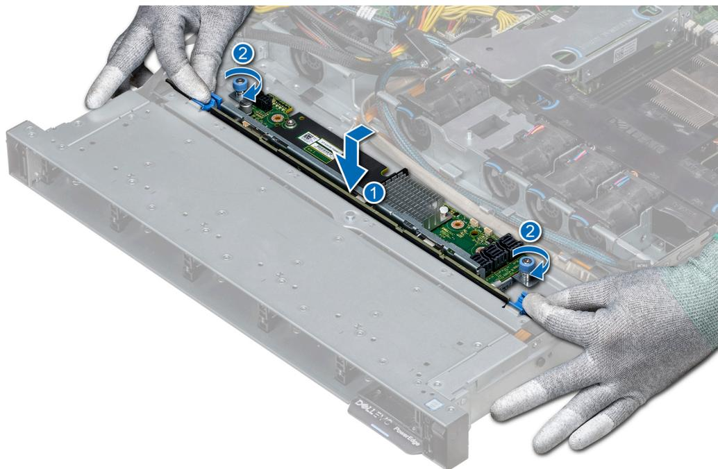
**Figure 87. Installing the hard drive backplane**
