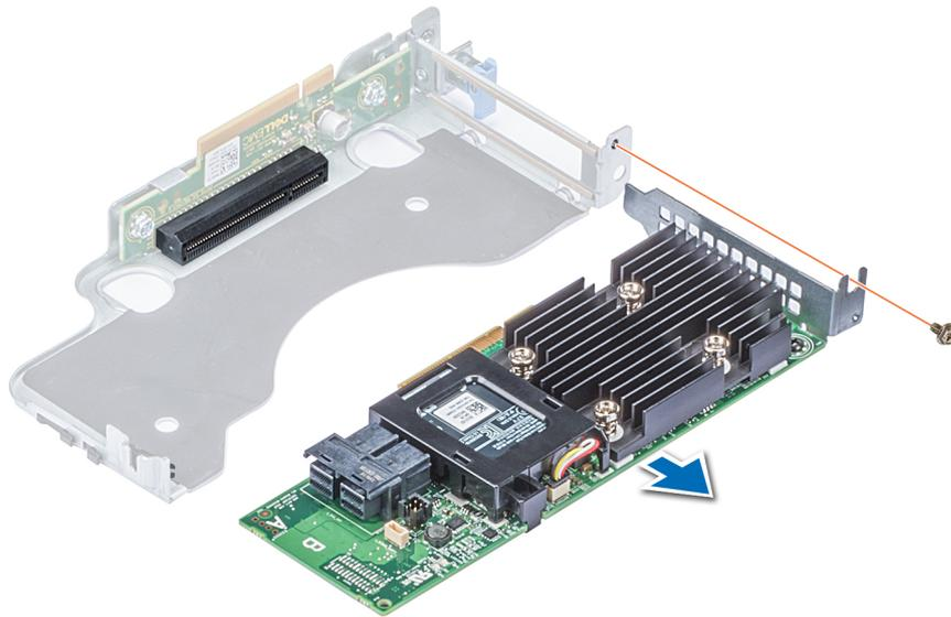
**Figure 73. Removing the PERC card from the internal PERC riser**
