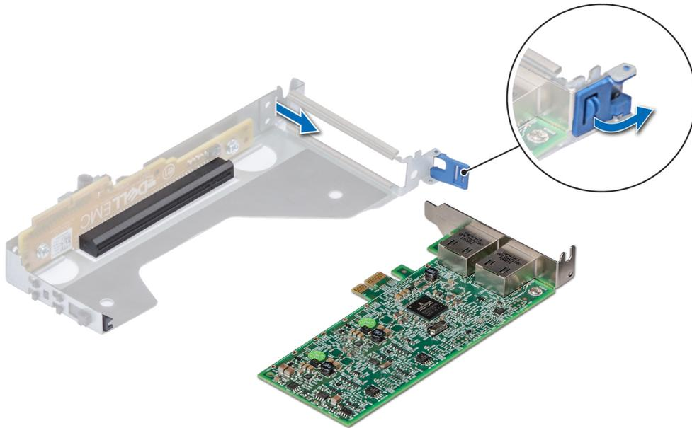
Figure 61. Removing expansion card from riser 2
