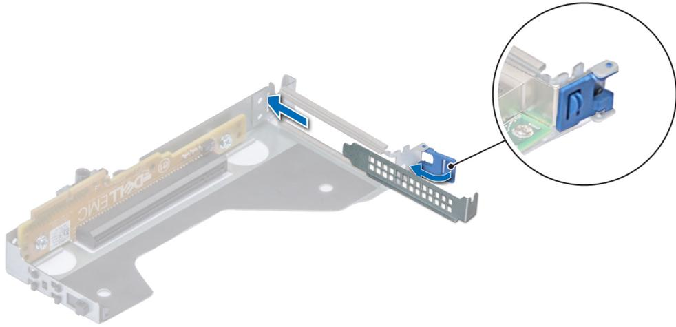
Figure 63. Installing filler bracket for riser 2
