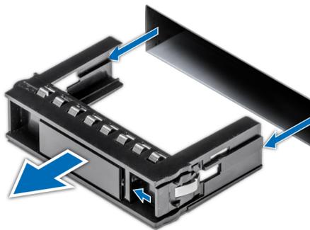
Figure 30. Removing a drive blank
