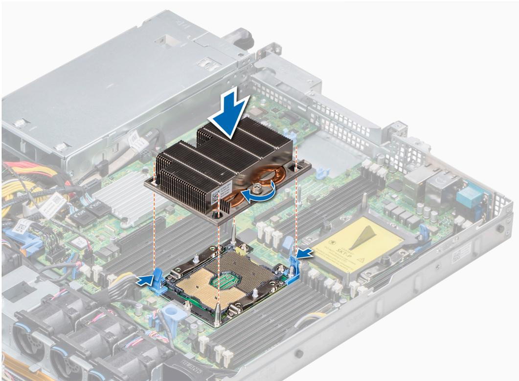
**Figure 44. Installing the processor and heat sink module**
