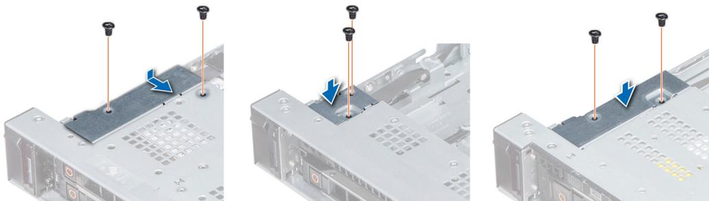
**Figure 107. Installing the cable cover**
