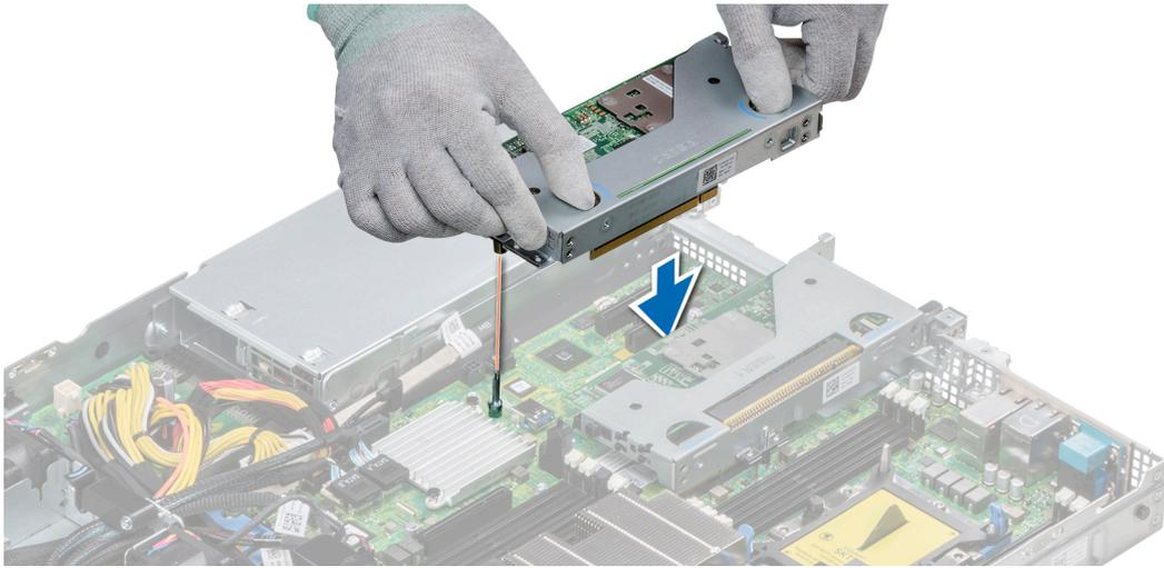
Figure 57. Installing an expansion card riser 2
