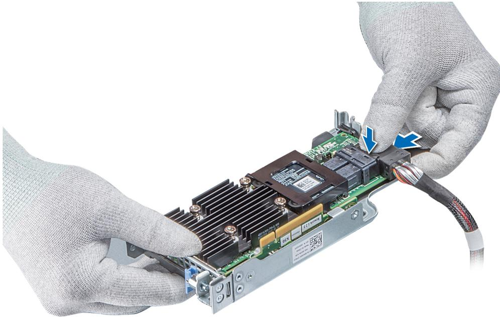
**Figure 51. Connecting the cable to internal PERC riser**
