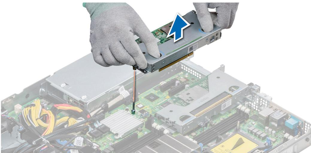
Figure 60. Removing an expansion card riser 2
