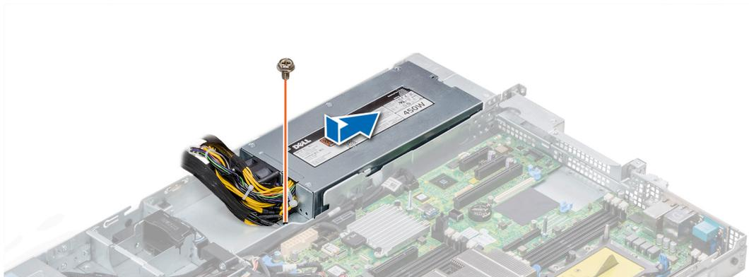
**Figure 102. Installing a non-redundant cabled AC PSU**
