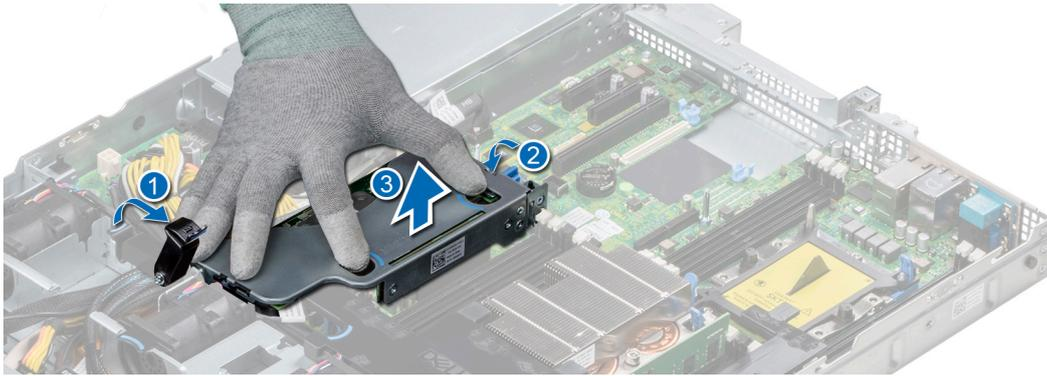
**Figure 69. Removing internal PERC riser**
