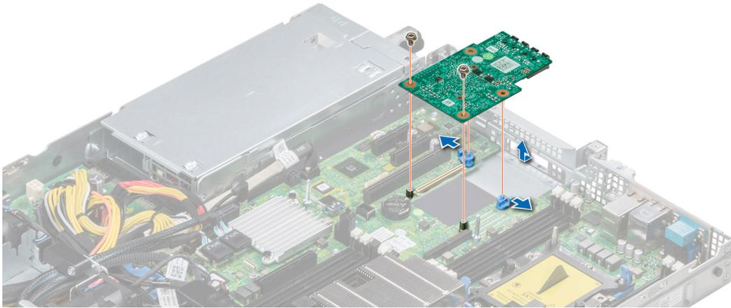
**Figure 81. Removing LOM riser card**
