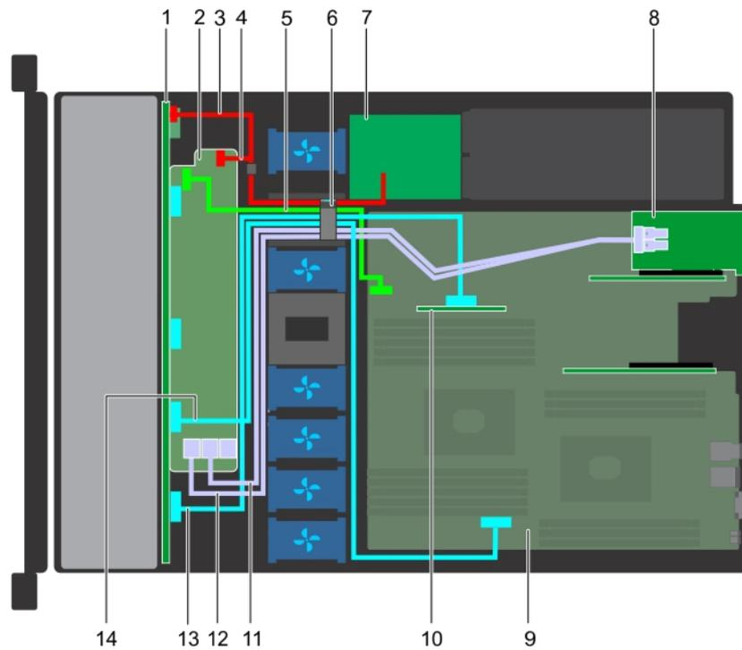
**Figure 90. Cable routing - 10 x 2.5 hard drive backplane with NVMe**
