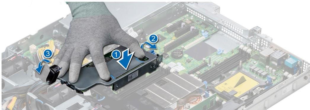
**Figure 72. Installing internal PERC riser**
