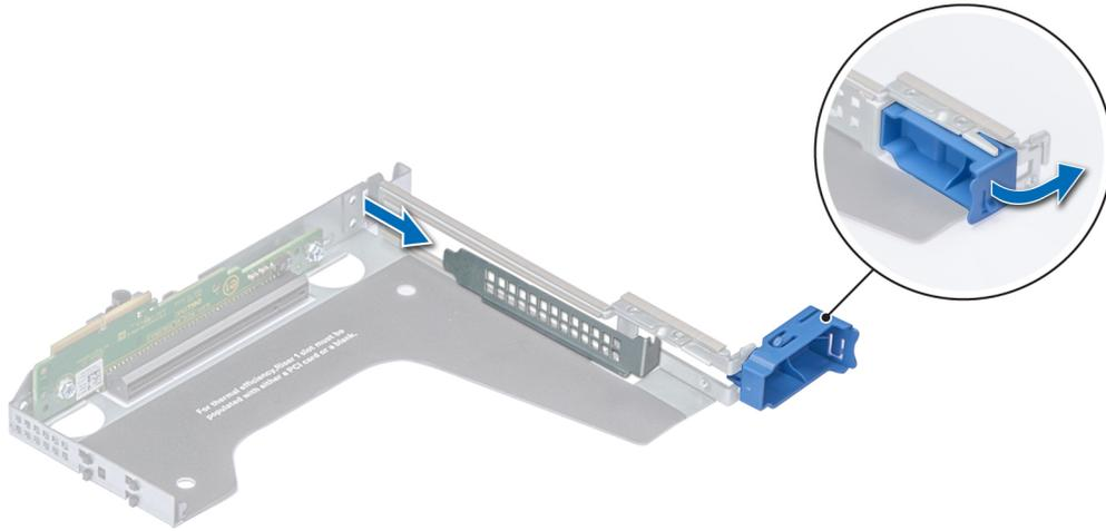
**Figure 66. Removing filler bracket for riser 1**
