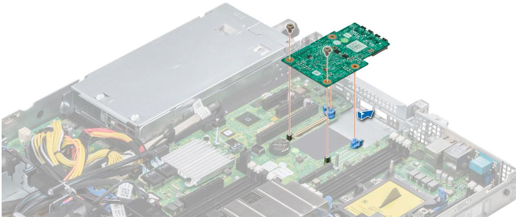
**Figure 82. Installing LOM riser card**
