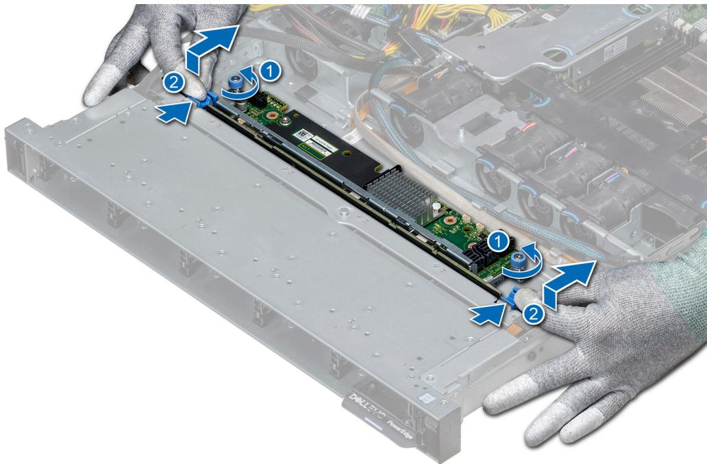
**Figure 88. Removing the hard drive backplane**
