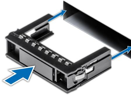
**Figure 31. Installing a drive blank**
