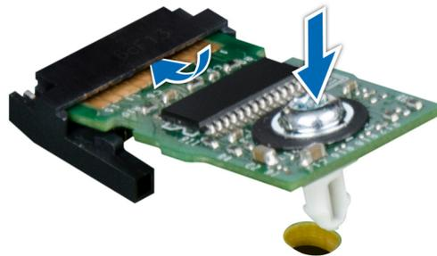
Figure 113. Installing the TPM
