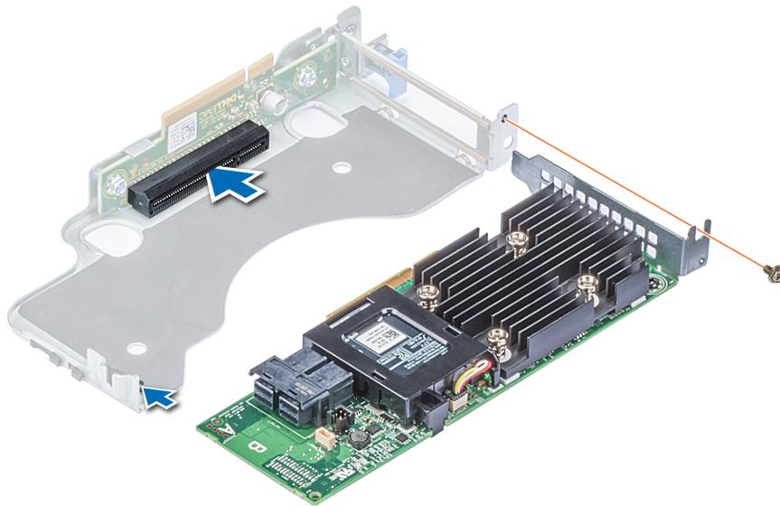
**Figure 74. Installing PERC card into internal PERC riser**
