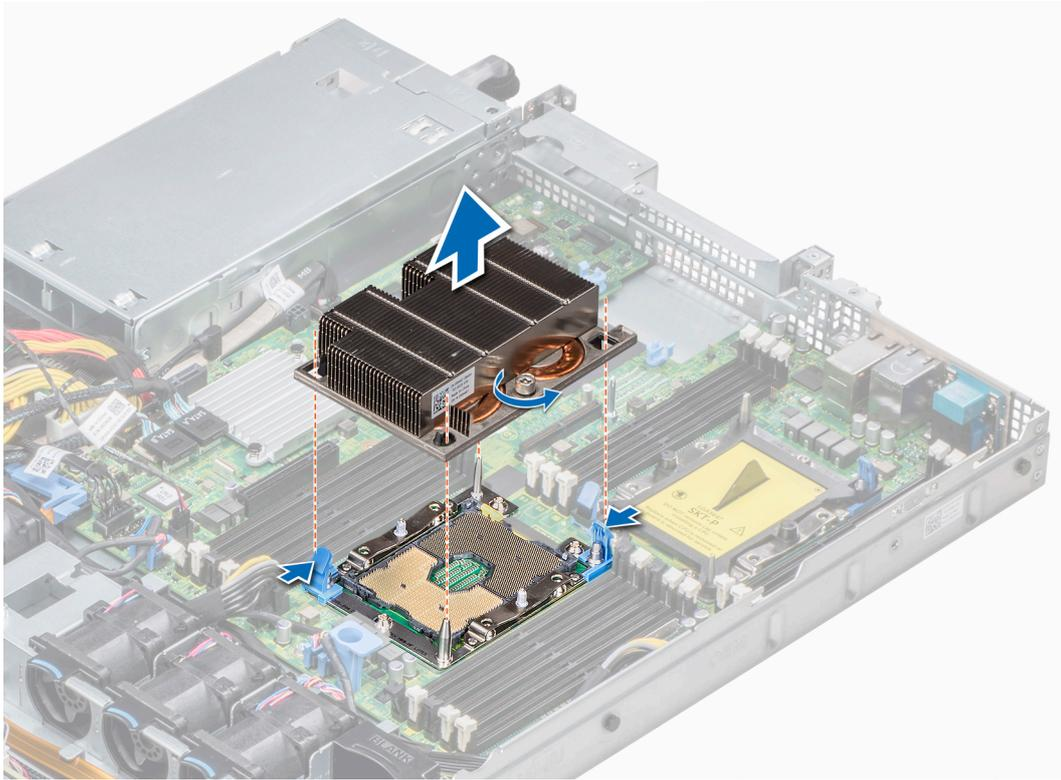
Figure 43. Removing processor and heat sink module
