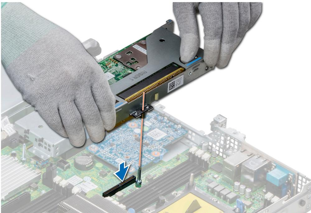
Figure 56. Installing an expansion card riser 1
