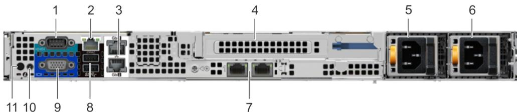
**Figure 9. Back view of the system with full height riser**
