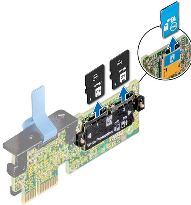
Figure 77. Removing the MicroSD card
