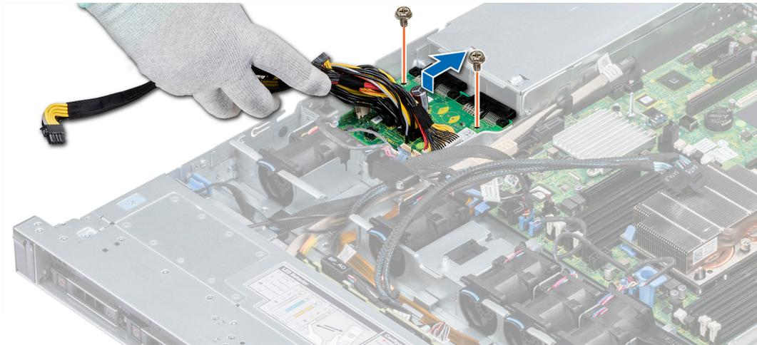
**Figure 103. Removing power interposer board**
