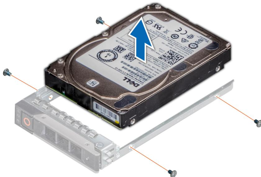
Figure 38. Removing the drive from the drive carrier
