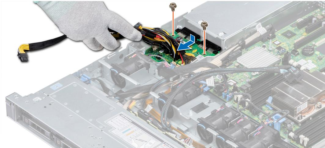
Figure 104. Installing power interposer board
