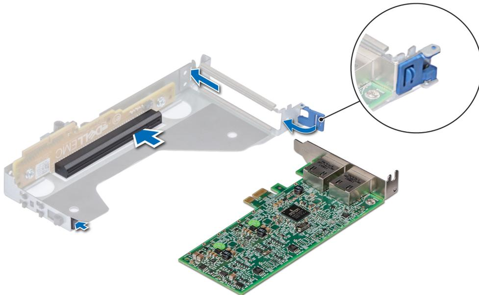
**Figure 67. Installing expansion card into riser 2**
