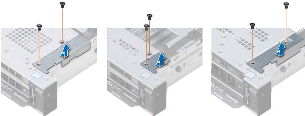
**Figure 108. Removing the cable cover**
