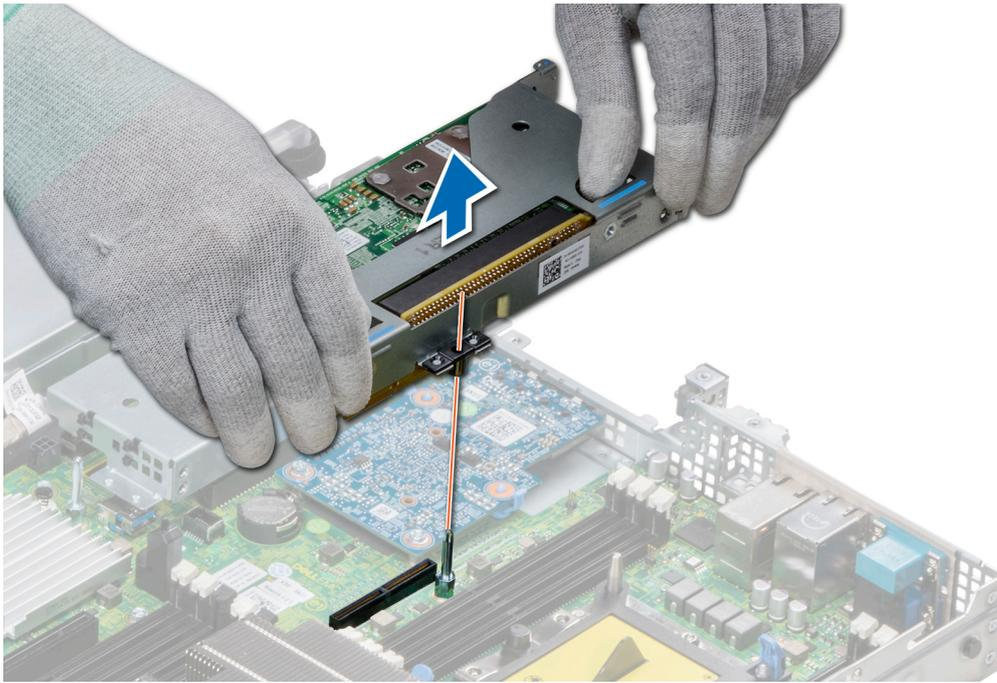
Figure 59. Removing an expansion card riser 1
