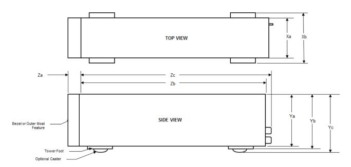
Figure 1. Dimensions of the Dell EMC PowerEdge T640 system
