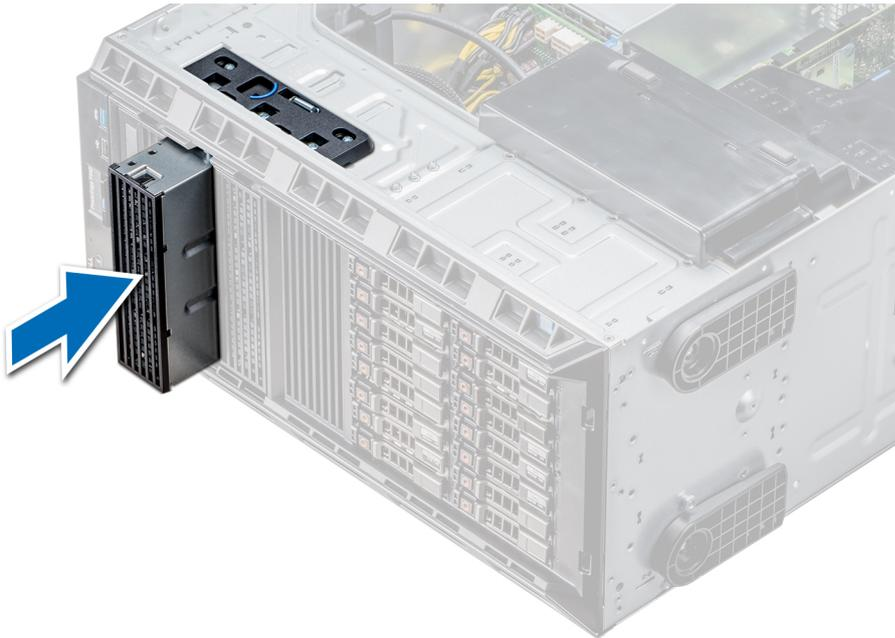
**Figure 38. Installing the optical or tape drive blank**
