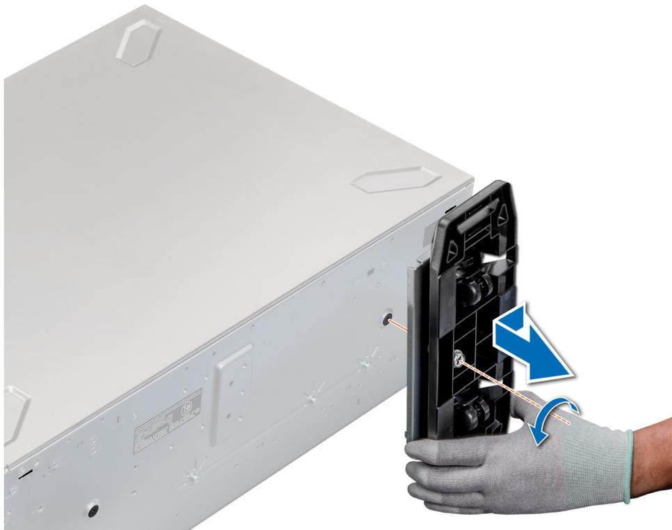
Figure 21. Removing caster wheels
