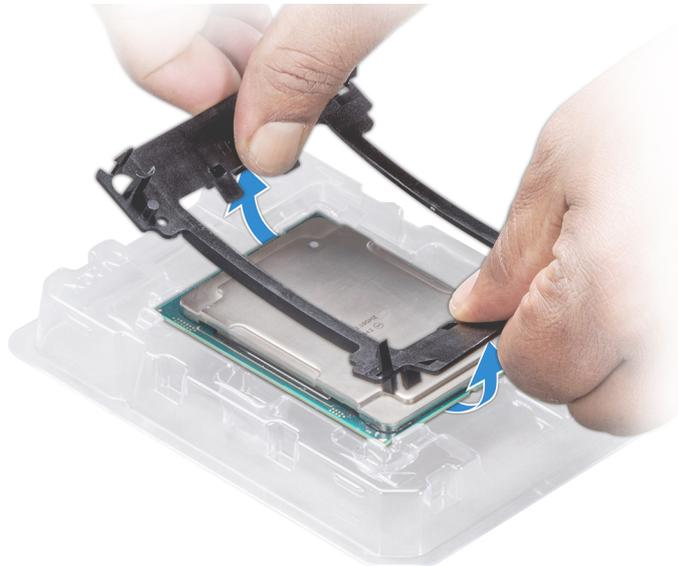
**Figure 74. Removing the processor bracket**
