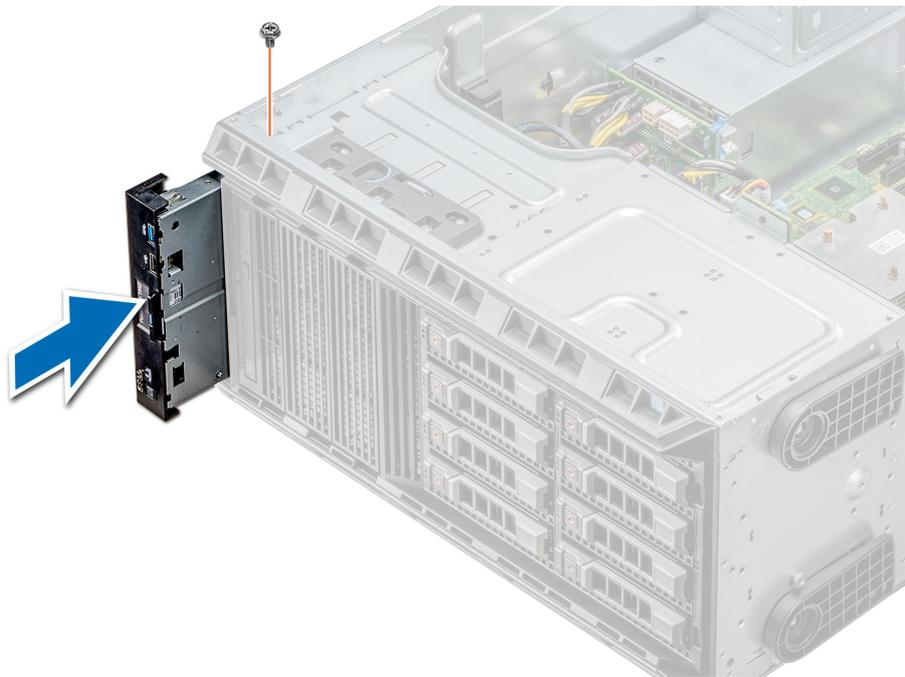
**Figure 91. Installing the control panel assembly**
