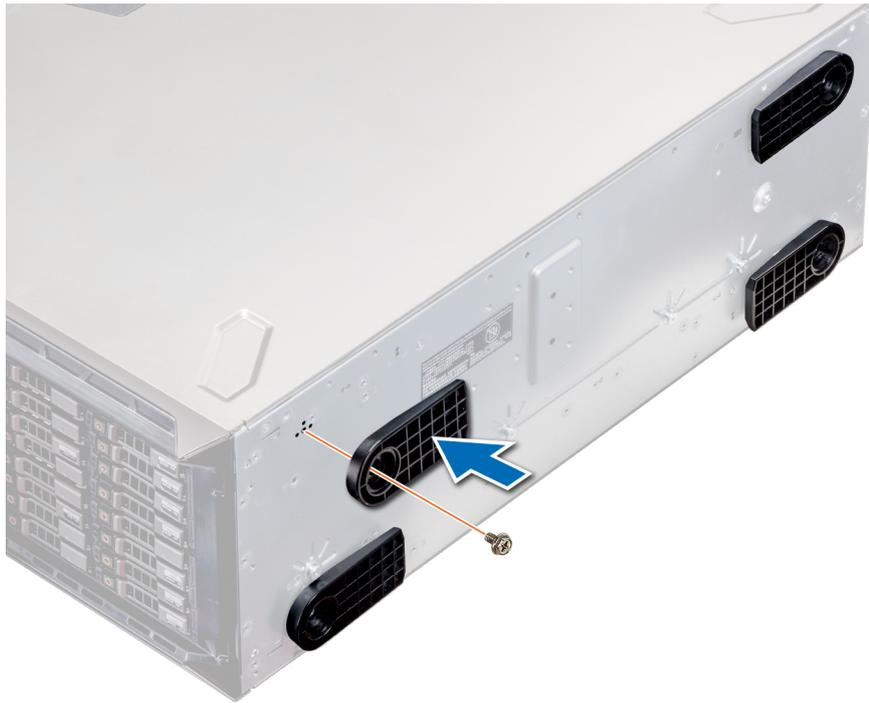
**Figure 18. Installing the system feet**
