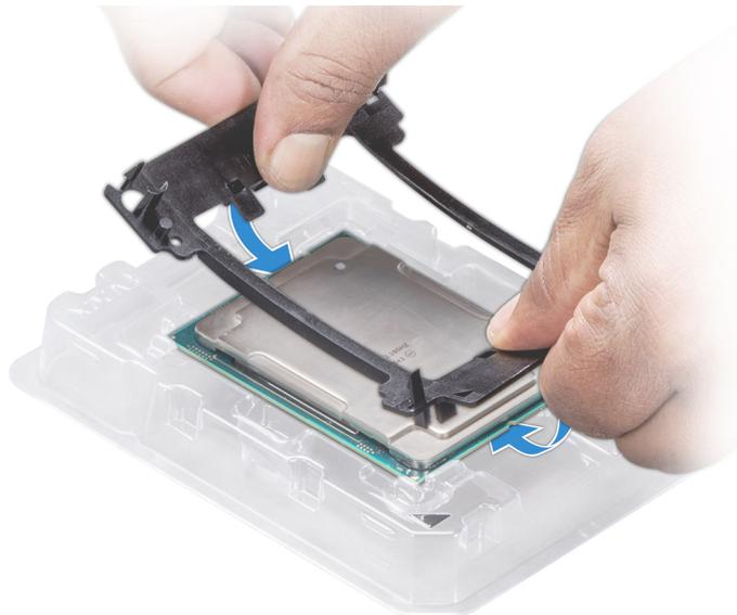
**Figure 75. Installing the processor bracket**
