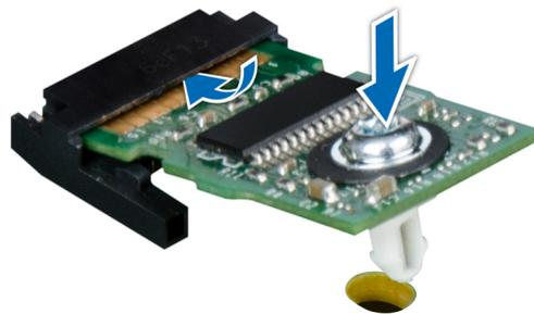
Figure 95. Installing the TPM
