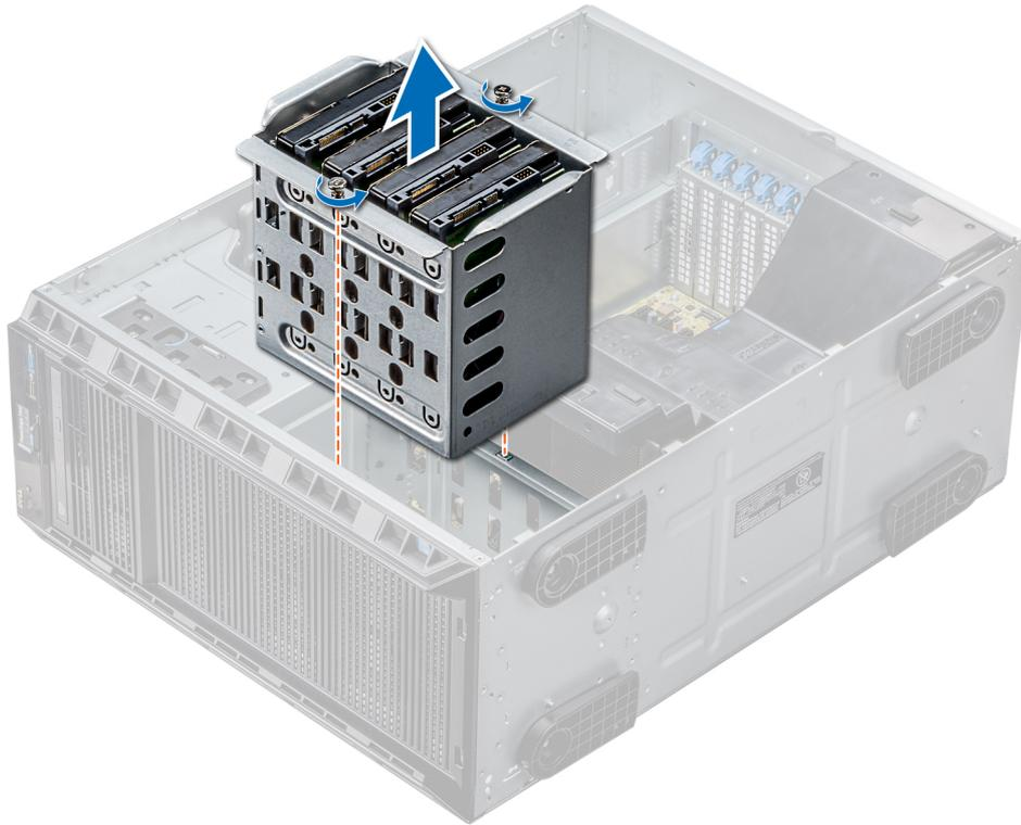
**Figure 41. Removing the internal hard drive bay**
