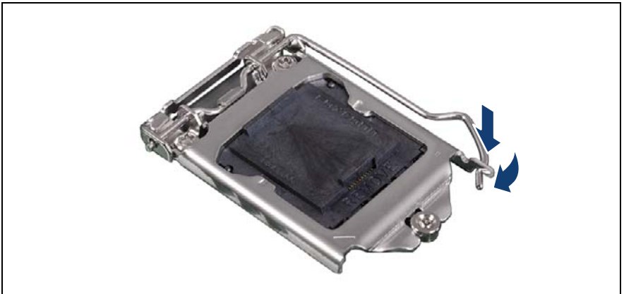
Figure 232: Latching the socket lever
