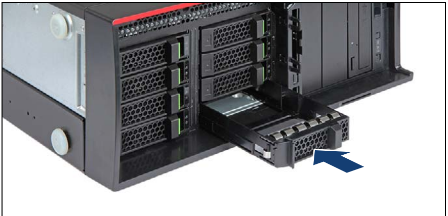
Figure 101: Installing a 3.5-inch HDD dummy module
