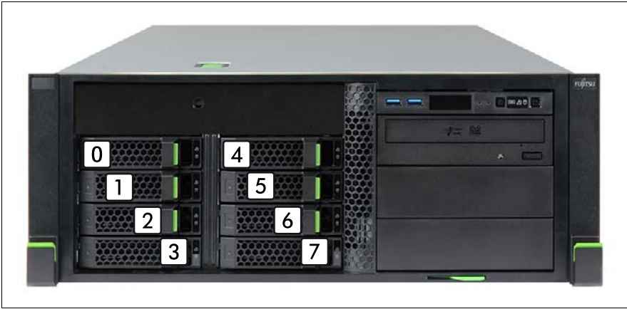
Figure 95: Configuration with up to eight 3.5-inch HDDs
