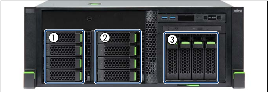
Figure 92: 3.5-inch HDD SAS backplanes - rack model
