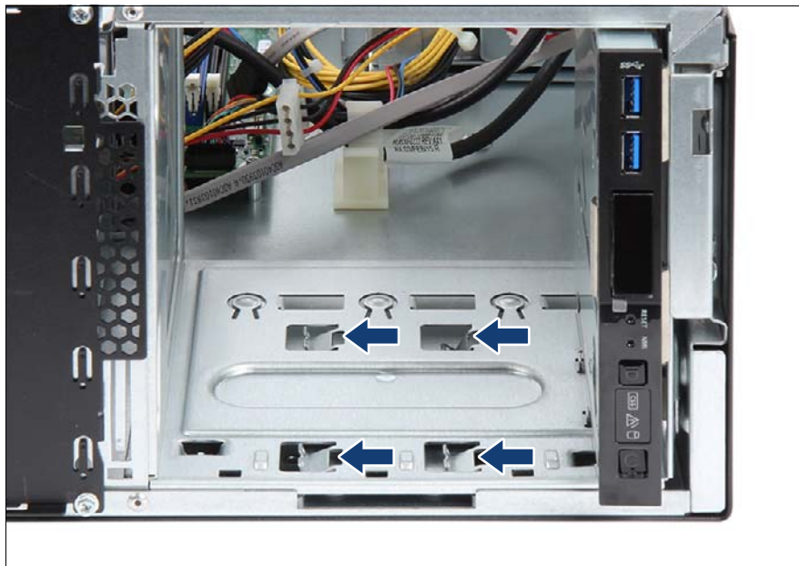
Figure 155: Bending in mounting brackets
