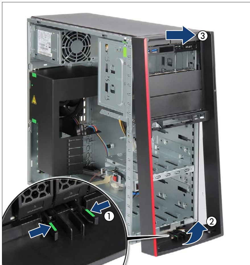
Figure 19: Removing the front cover (floorstand model)
