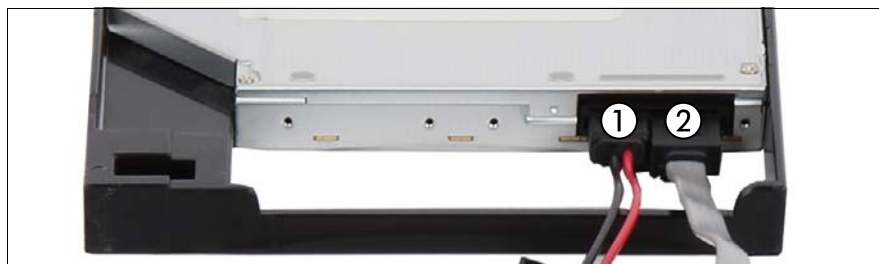
Figure 251: Connecting cables to the slimline ODD
