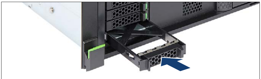
Figure 125: Installing a 2.5-inch HDD/SSD dummy module
