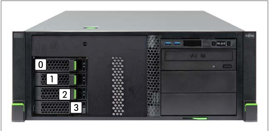
Figure 94: Configuration with up to four 3.5-inch HDDs
