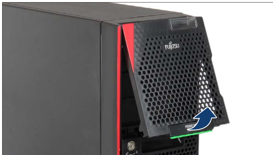
Figure 15: Removing the accessible drive bay cover
