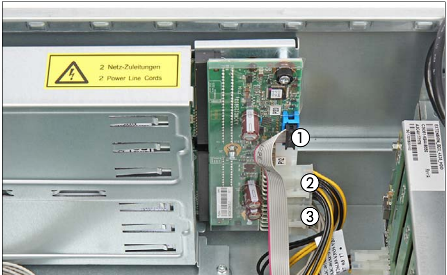
Figure 78: Connecting the power distribution board
