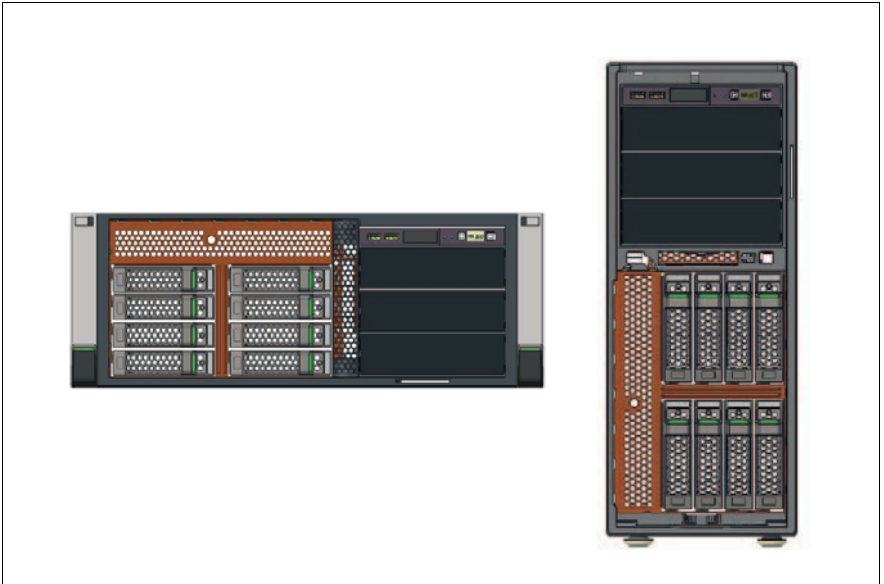
Figure 84: Rack model versus floorstand model with drive cage turned
