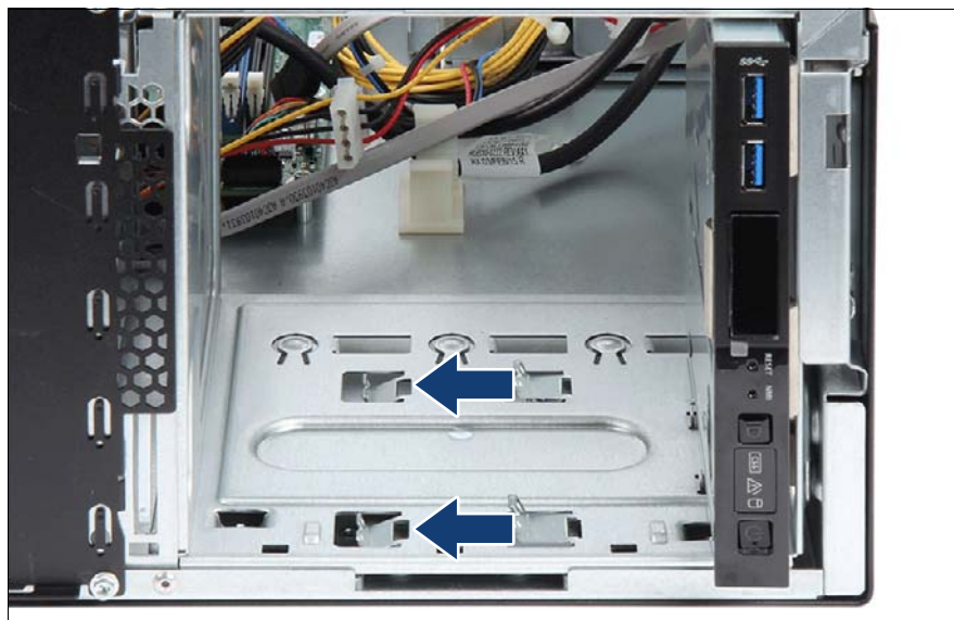
Figure 144: Bending in mounting brackets
