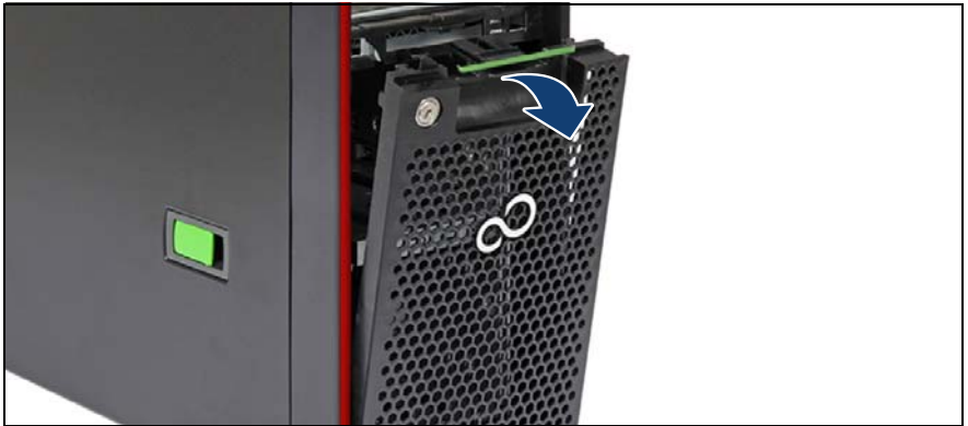
Figure 17: Removing the HDD bay cover
