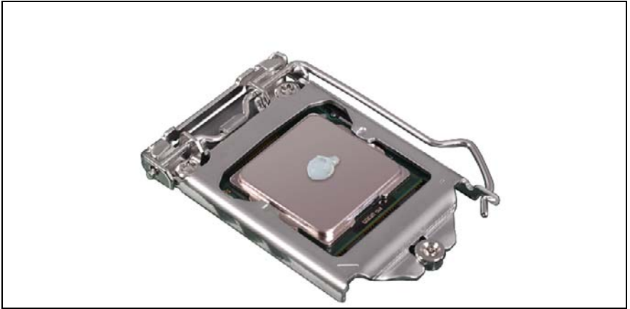
Figure 227: Applying thermal paste
