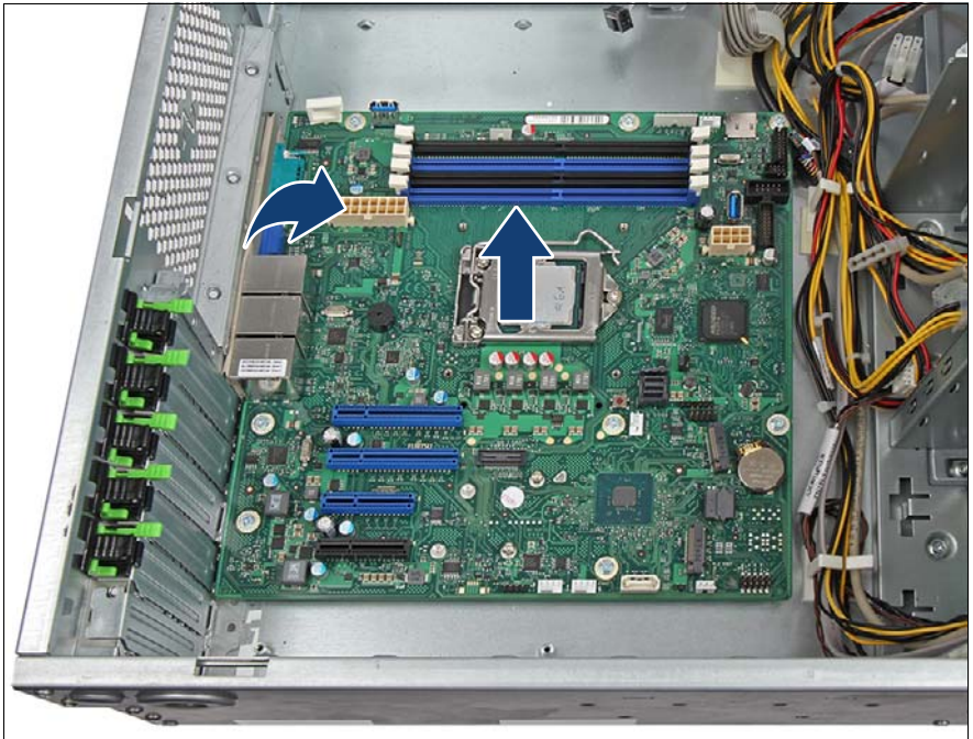
Figure 298: Removing the system board
