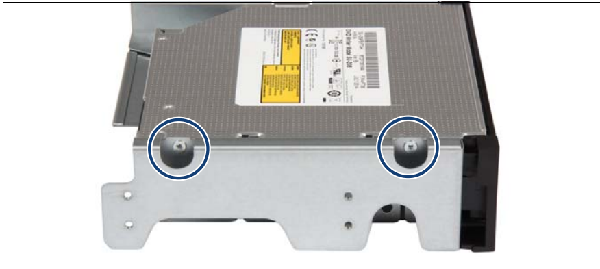
Figure 265: Installing the ultraslim ODD in the ultraslim ODD adapter (B)
