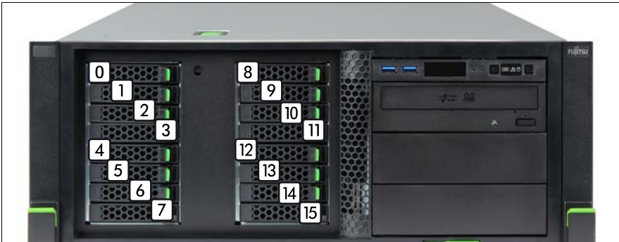
Figure 119: Configuration with up to 16 2.5-inch HDDs/SSDs
