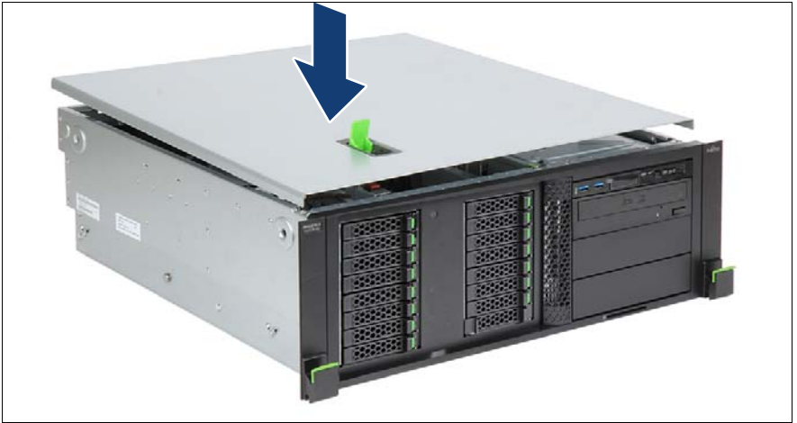
Figure 23: Installing the top cover (rack server) (A)
