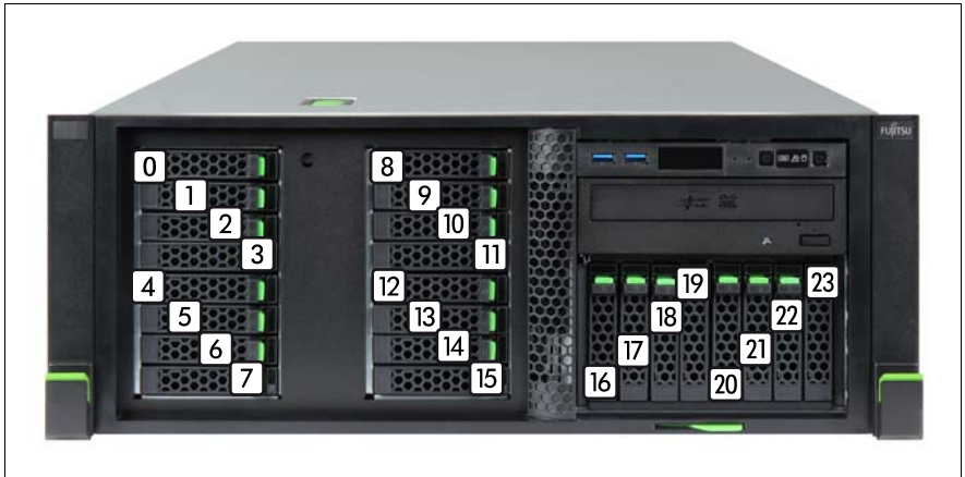
Figure 120: Configuration with up to 24 2.5-inch HDDs/SSDs with HDD extension box
