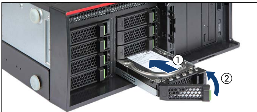
Figure 100: Installing the 3.5-inch HDD module
