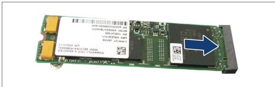
Figure 287: Installing the M.2 SSD
