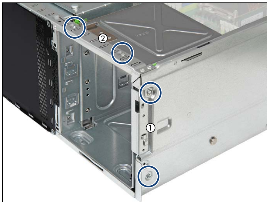
Figure 309: Securing the accessible drive cage (A)
