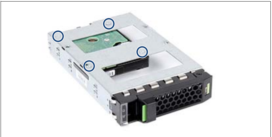
Figure 89: Installing the 2.5-inch HDD/SSD in the 3.5-inch installation frame (B)
