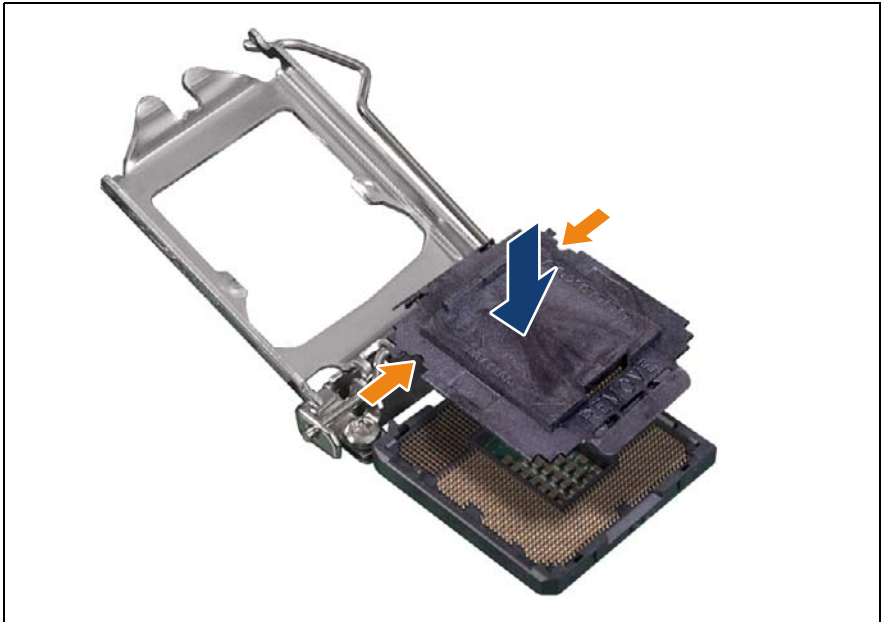
Figure 229: Attaching the protective socket cover
