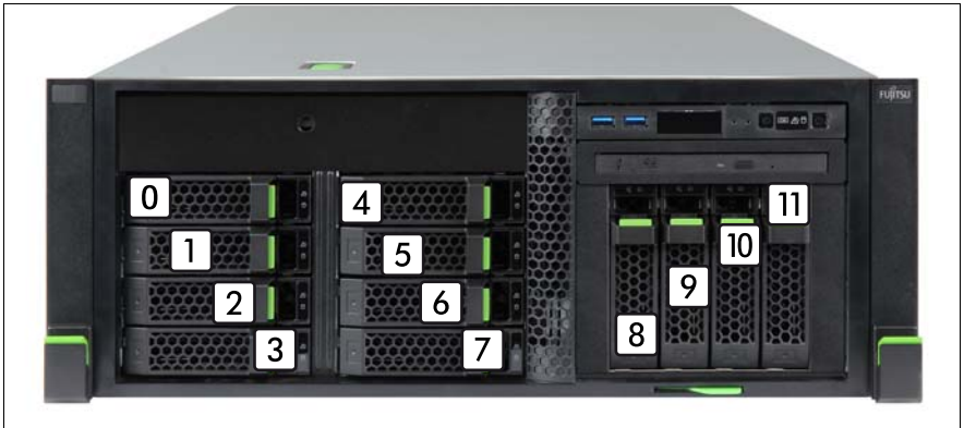
Figure 96: Configuration with up to 12 3.5-inch HDDs
