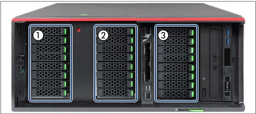
Figure 117: Example three backplanes - floorstand model
