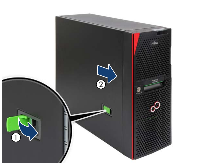
Figure 32: Installing the side cover (floorstand model)
