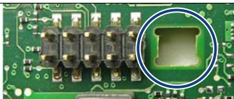
Figure 276: Position for the TPM spacer
