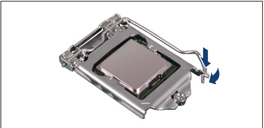
Figure 225: Closing the socket release lever
