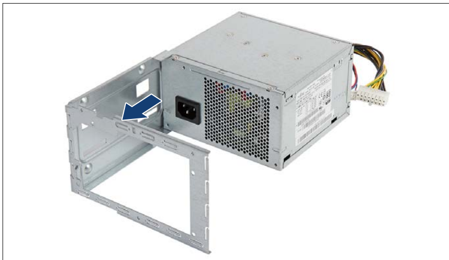
Figure 60: Removing the installation frame from the PSU (B)
