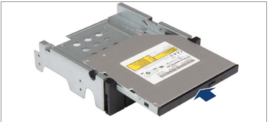
Figure 264: Installing the ultraslim ODD in the ultraslim ODD adapter (A)
