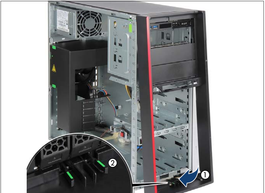
Figure 28: Installing the front cover (B)
