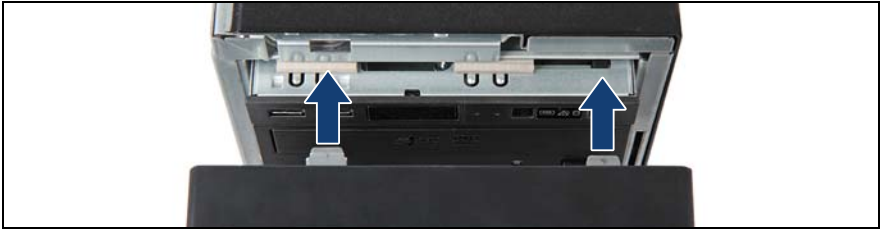
Figure 27: Installing the front cover (A)
