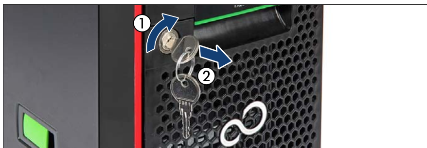
Figure 13: Unlocking the server
