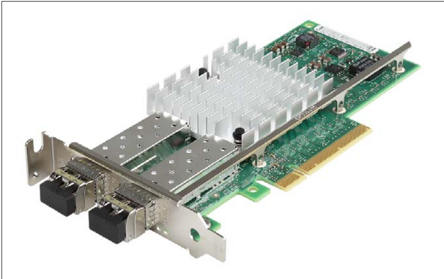
Figure 186: Installing the secondary SFP+ transceiver module
