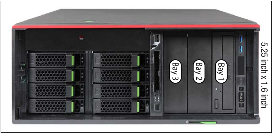
Figure 237: Accessible drives mounting order (floorstand model)
