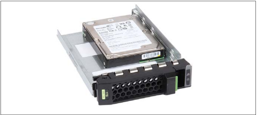
Figure 88: Installing the 2.5-inch HDD/SSD in the 3.5-inch installation frame (A)
