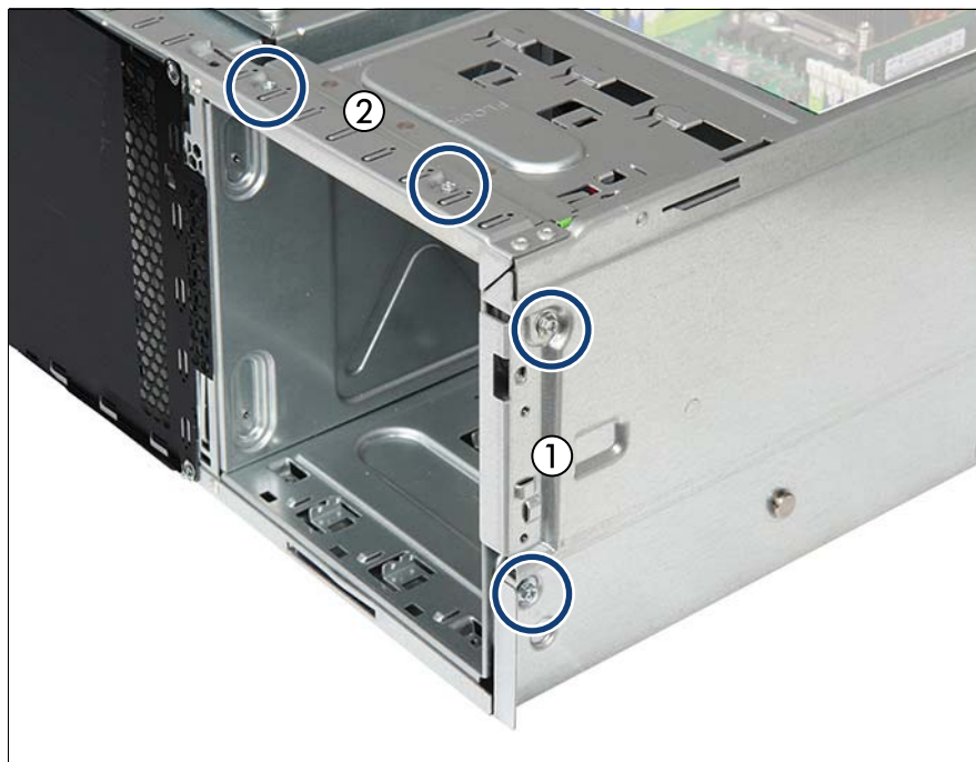
Figure 305: Detaching the accessible drive cage (B)
