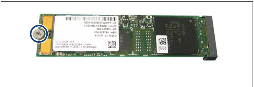
Figure 289: Removing the M.2 SSD (A)
