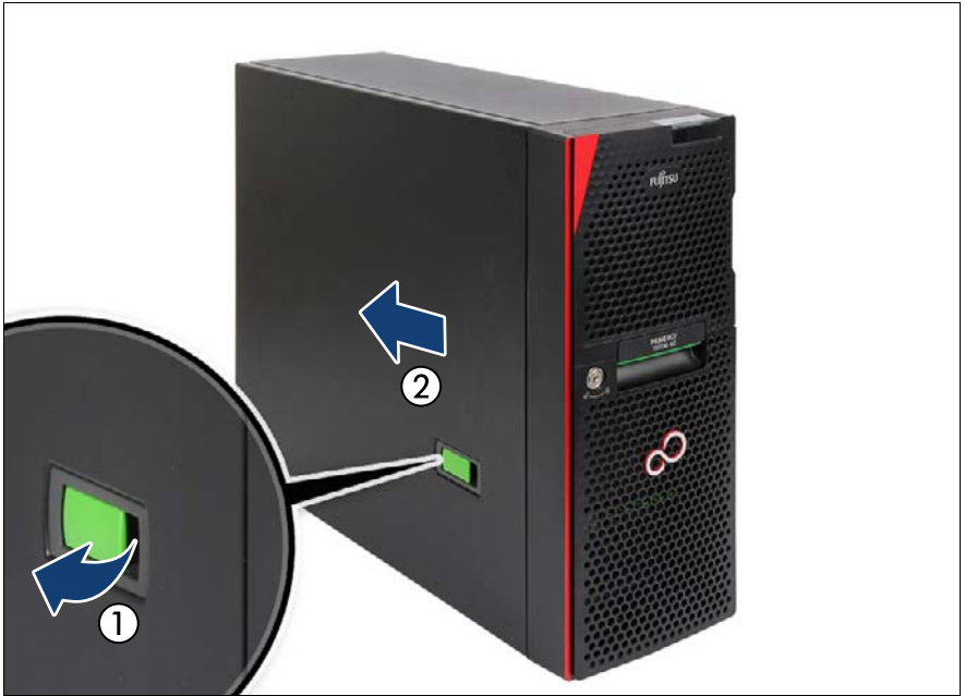
Figure 14: Removing the side cover (floorstand model)
