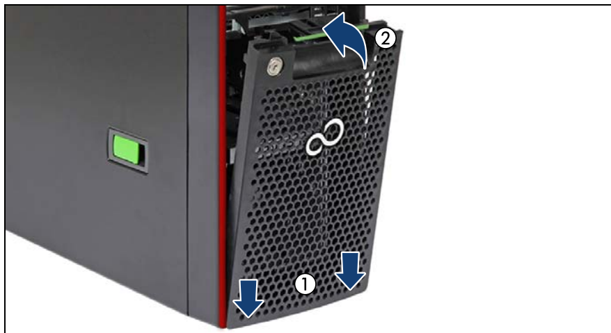
Figure 30: Installing the HDD bay cover
