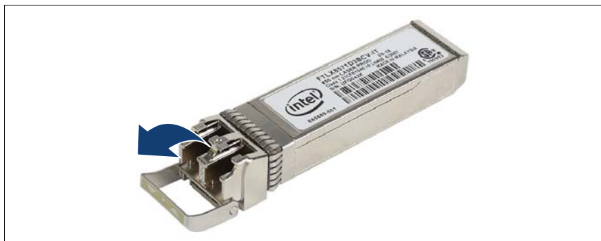
Figure 182: Unlatching the locking bail
