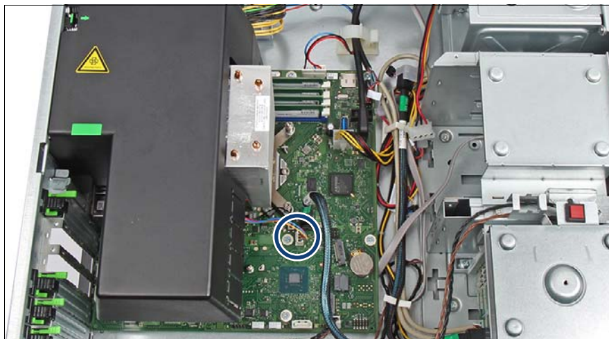
Figure 42: Connecting the system fan cable
