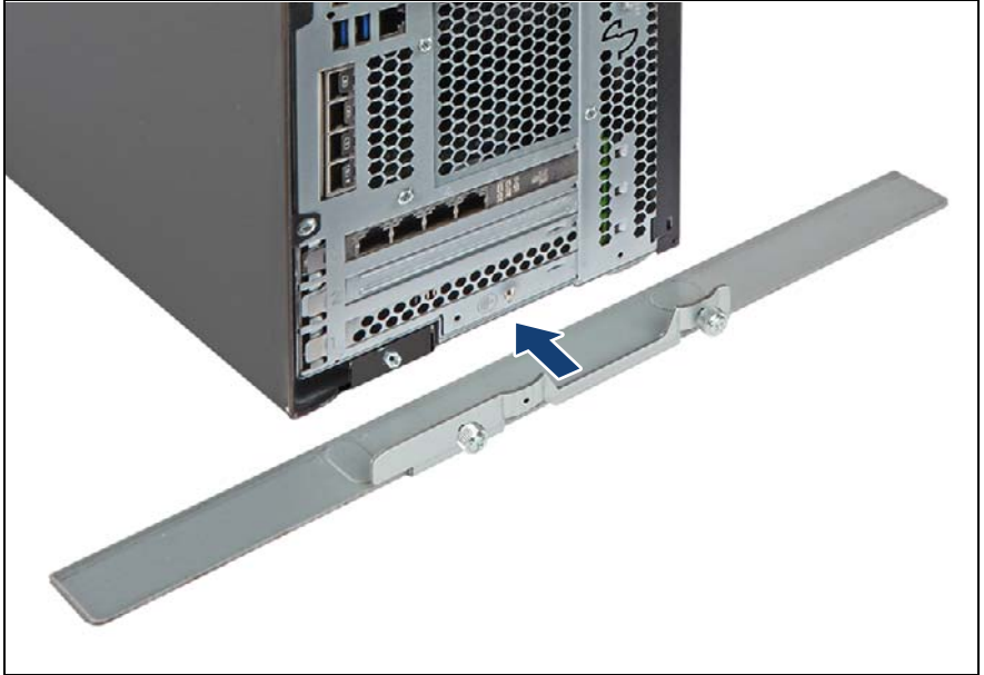
Figure 53: Installing the anti-tilt bracket (A)
