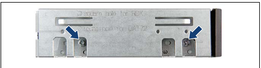
Figure 241: Securing mounting brackets to an RDX backup drive
