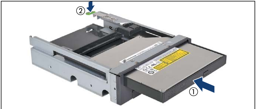
Figure 249: Mounting the slimline ODD module in the Multibay box
