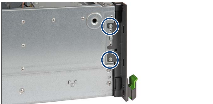
Figure 9: Removing the rack front cover (A)
