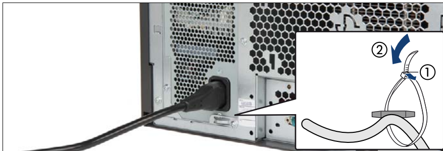
Figure 2: Unlocking the cable tie of a standard PSU
