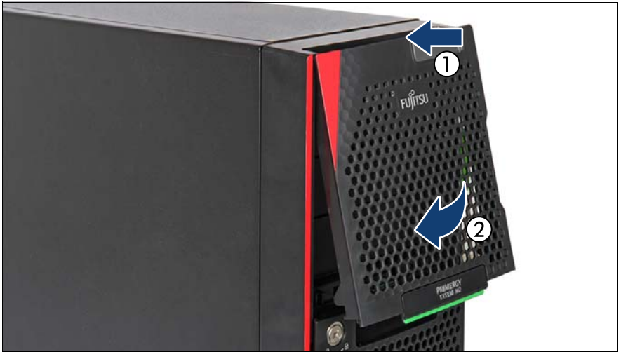
Figure 31: Installing the accessible drive bay cover
