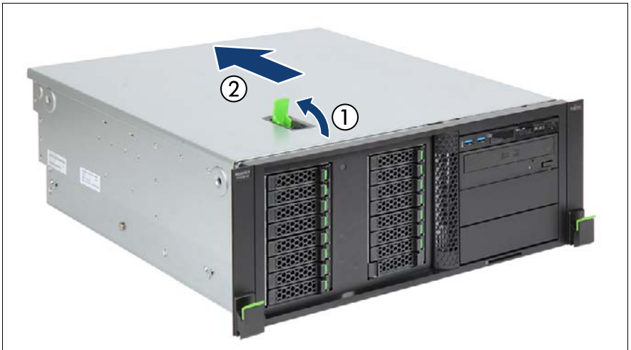
Figure 6: Removing the top cover (rack server)
