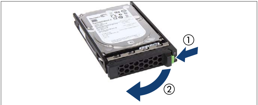
Figure 123: Opening the locking lever
