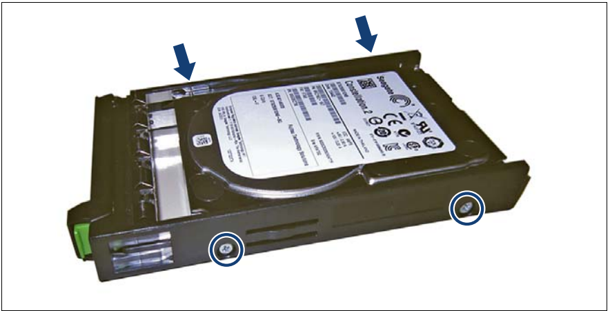
Figure 86: Installing the 2.5-inch HDD/SSD in the 2.5-inch installation frame (B)
