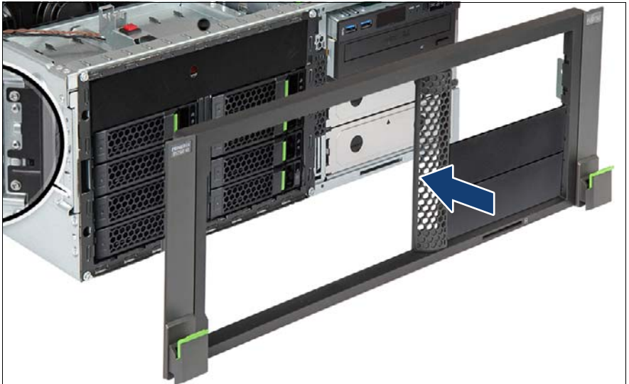
Figure 20: Installing the rack front cover
