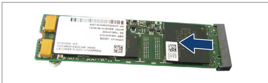
Figure 290: Removing the M.2 SSD (B)
