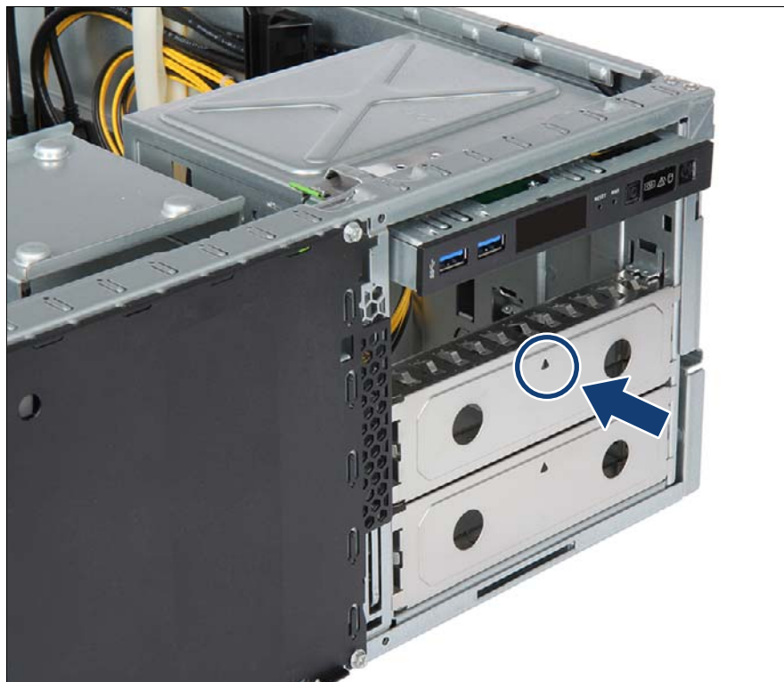
Figure 50: Installing an accessible drive filler cover
