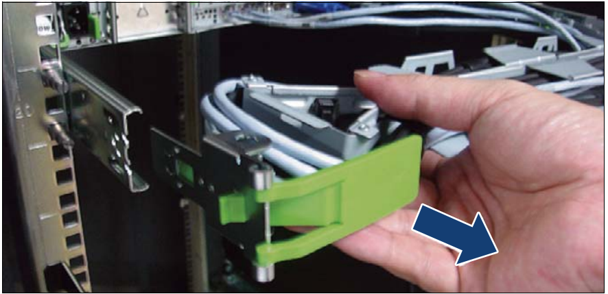
Figure 71: Removing the CMA stopper
