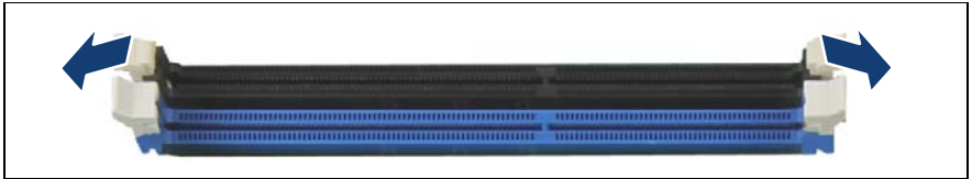
Figure 213: Opening the securing clips
