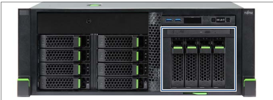
Figure 143: 4x 3.5-inch HDD extension box
