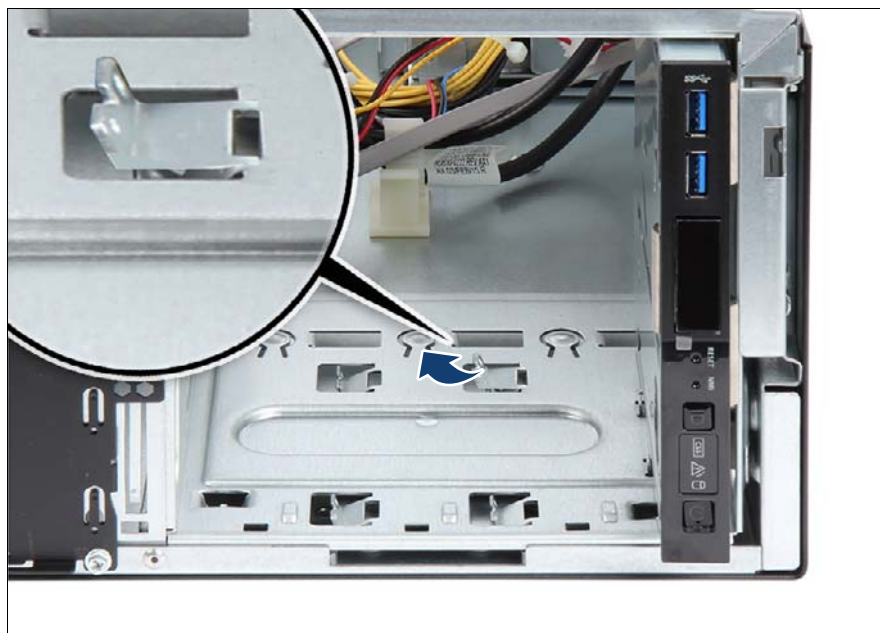
Figure 242: Mounting brackets in right position
