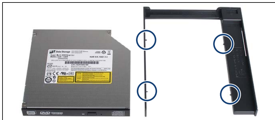
Figure 248: Mounting the slimline ODD in the installation frame
