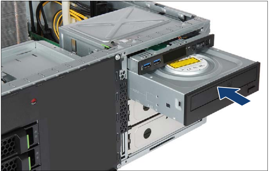
Figure 243: Inserting the accessible drive
