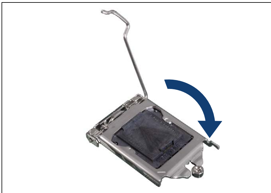
Figure 230: Closing the load plate (A)
