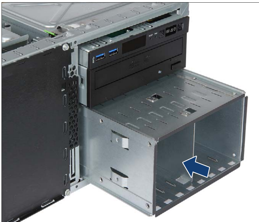
Figure 145: Inserting the 8x 2.5-inch HDD/SSD extension box
