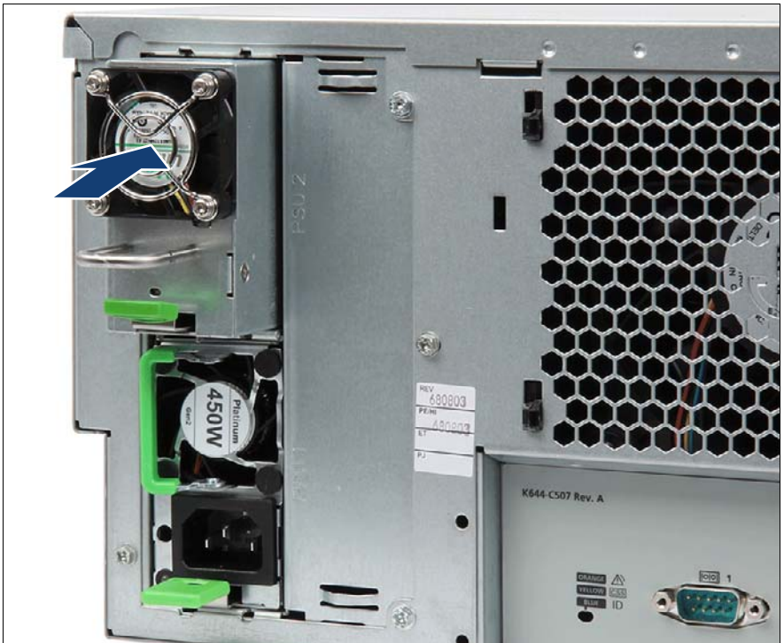
Figure 79: Installing a FJBU
