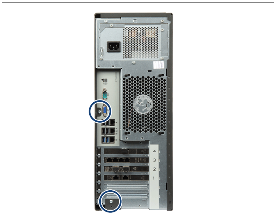
Figure 301: Removing the right side cover (A)
