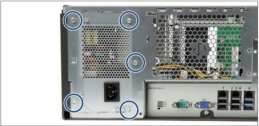
Figure 57: Removing the screws
