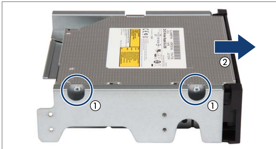
Figure 266: Removing the ultraslim ODD from the ultraslim ODD adapter
