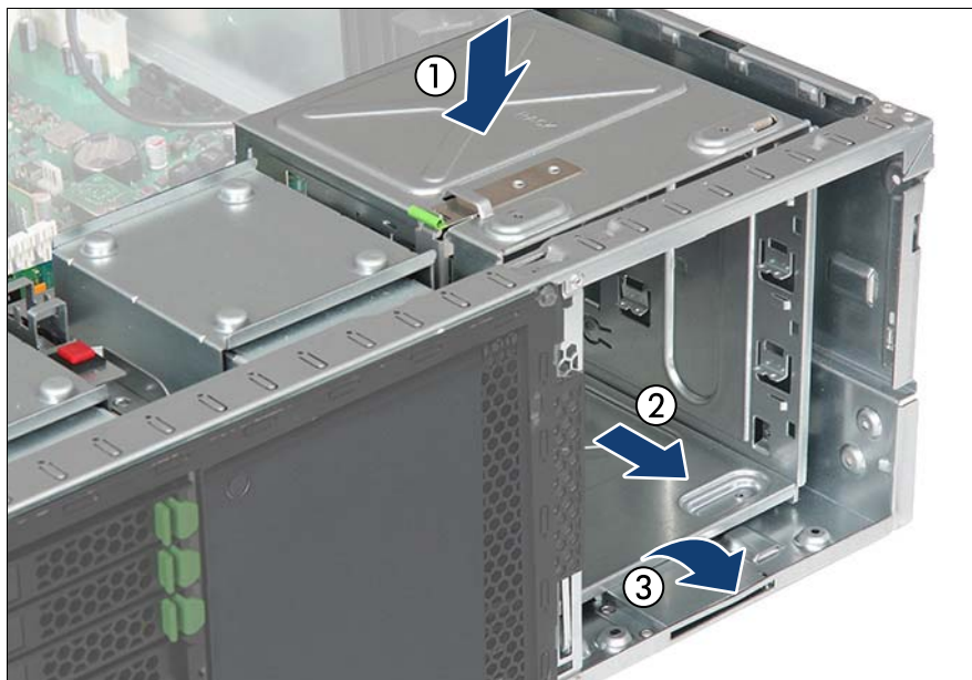
Figure 308: Mounting the accessible drive cage
