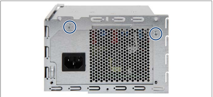
Figure 62: Securing the installation frame to the PSU
