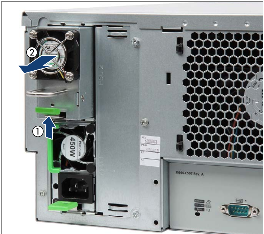
Figure 80: Removing a FJBU
