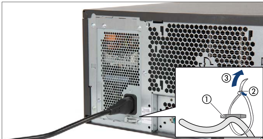
Figure 35: Securing power cord
