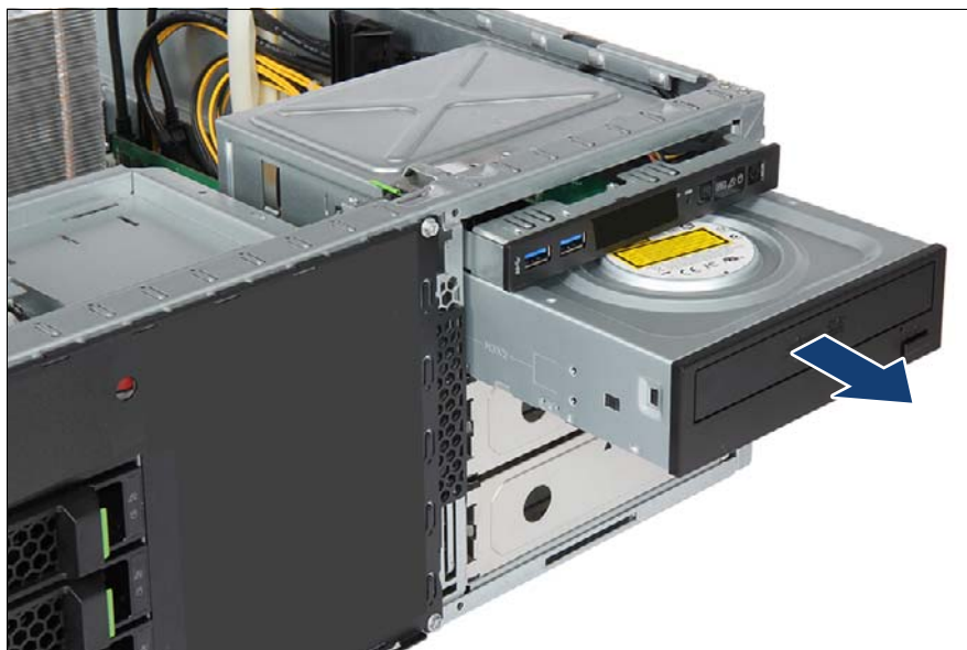
Figure 246: Removing the accessible drive
