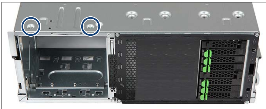
Figure 304: Detaching the accessible drive cage (A)
