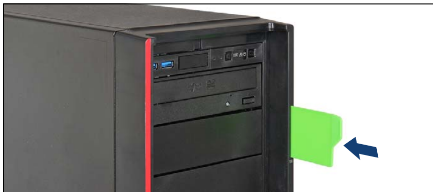
Figure 29: Installing the ID card (floorstand model)
