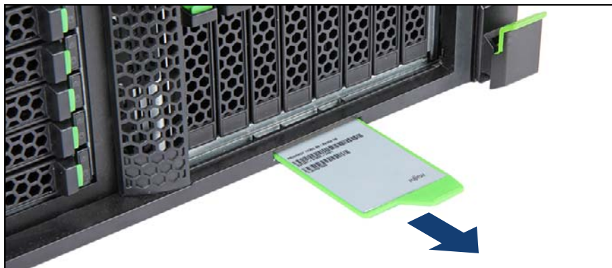
Figure 8: Removing the ID card (rack model)
