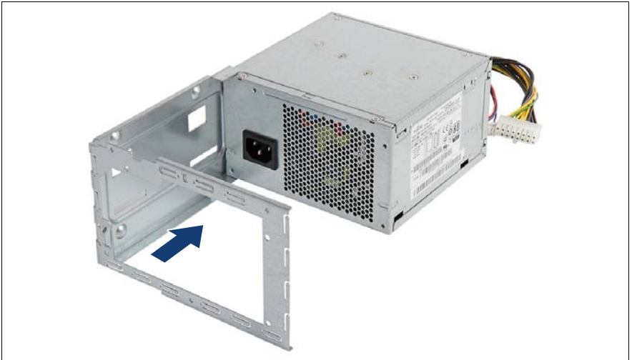
Figure 61: Attaching the installation frame to the PSU
