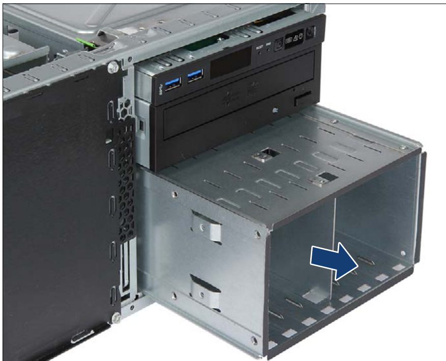
Figure 148: Removing the 8x 2.5-inch HDD/SSD extension box
