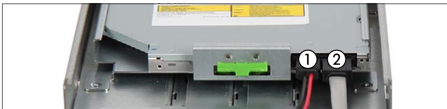
Figure 260: Connecting cables to the ultraslim ODD
