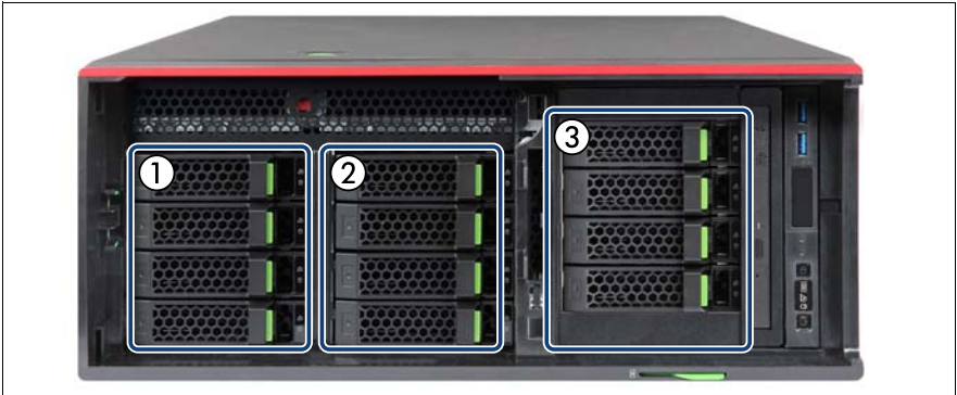
Figure 93: 3.5-inch HDD SAS backplanes - floorstand model
