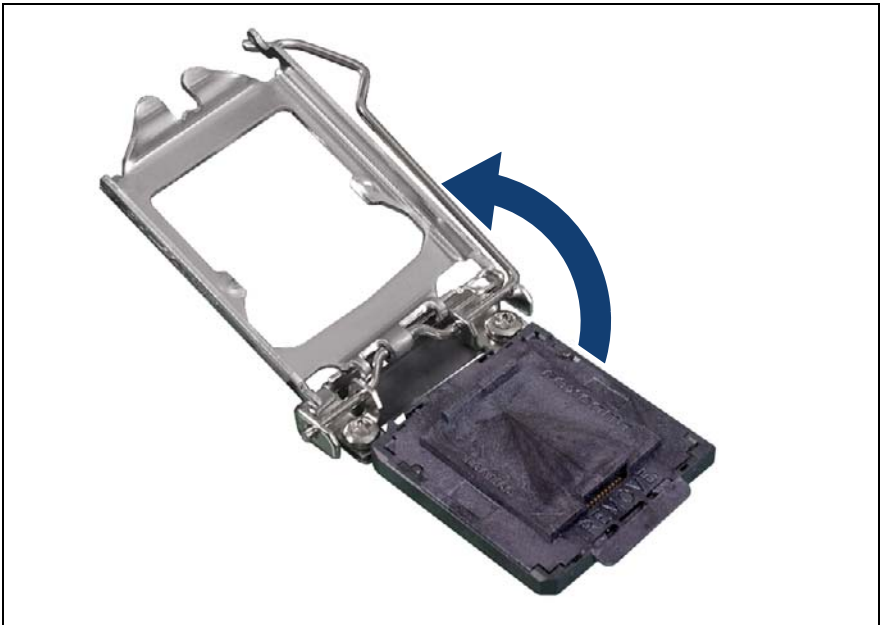
Figure 234: Opening the load plate
