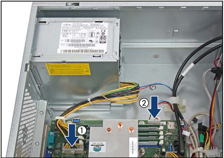
Figure 64: Connecting the power cables
