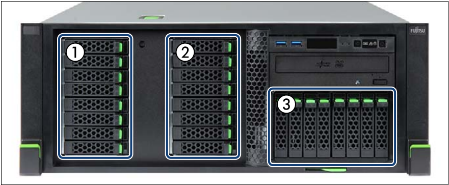
Figure 116: Example three backplanes - rack model
