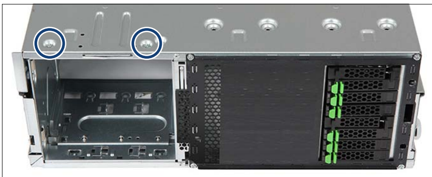
Figure 310: Securing the accessible drive cage (B)
