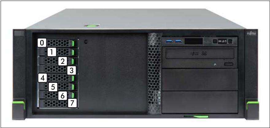
Figure 118: Configuration with up to eight 2.5-inch HDDs/SSDs
