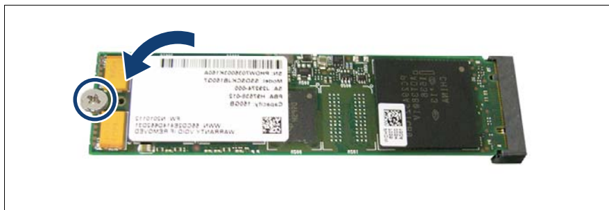
Figure 288: Fastening the M.2 SSD
