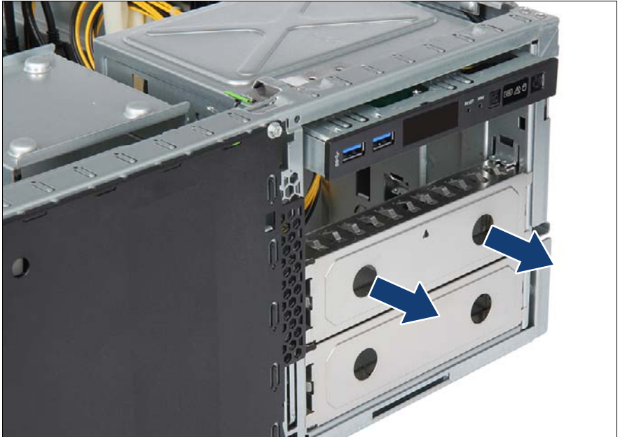
Figure 49: Removing an accessible drive filler cover
