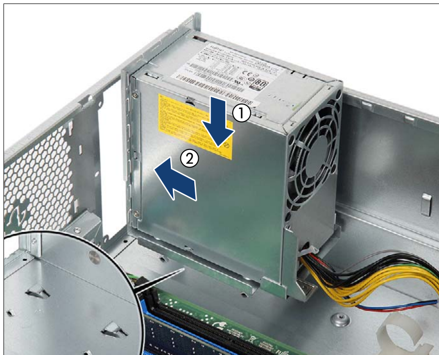
Figure 63: Installing the standard PSU
