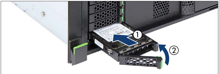
Figure 124: Installing the 2.5-inch HDD/SSD module
