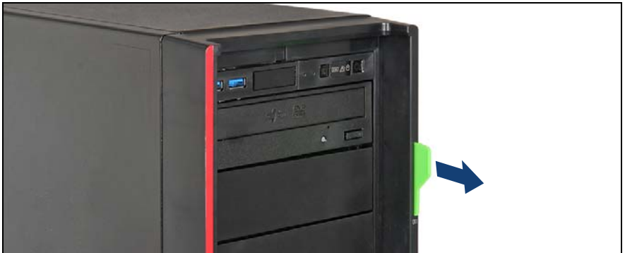
Figure 18: Removing the ID card (floorstand model)
