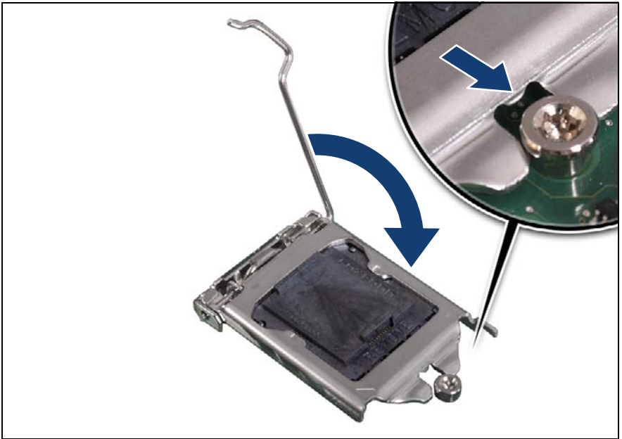
Figure 231: Closing the load plate (B)
