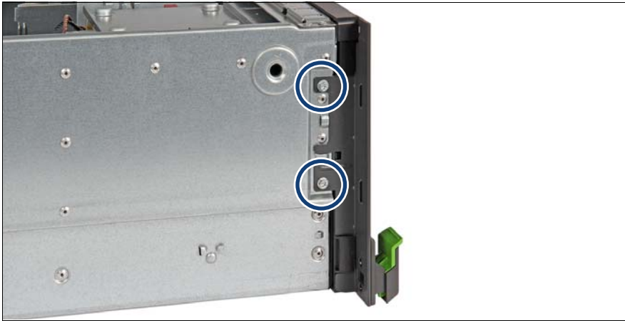
Figure 21: Installing the rack front cover (B)
