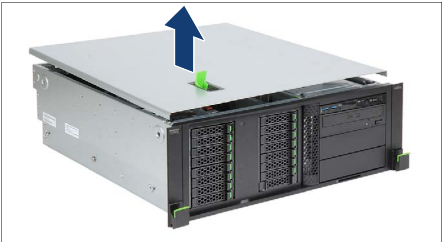
Figure 7: Removing the top cover (rack server)
