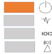
Figure: Power supply does not have redundancy
