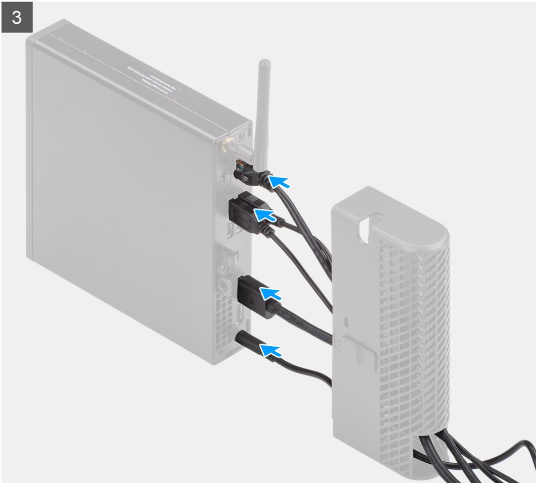
7. Align the cable cover retaining hooks into the slots on the OptiPlex 5080 Micro chassis.
