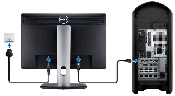
(i) NOTE: The DisplayPort on the back panel of your computer is covered. Connect the display to the discrete graphics card of your computer.
