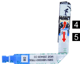
Figure 23. Remove the power board cable from power board
