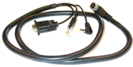
Image 9-3: Customized cable to connect Touch Panel interface with the Barco projector.
