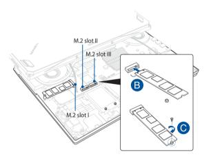
**NOTE:** The M.2 2280 slot II supports PCIe (NVMe) SSD while slot I and slot III support both PCIe (NVMe) SSD and SATA SSD.
