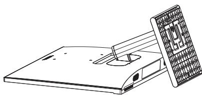
2. (1) Use a screwdriver to loosen the screw located at the bottom of the base.
