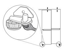
Open the door and use the spanner 10 to loosen the keeper nut by turning it to the left.
