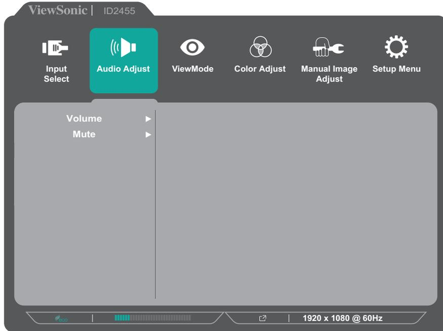
3. Press the **1(ViewMode)** or **2** key to select the desired option. Then press the **3** key to enter its sub-menu.
