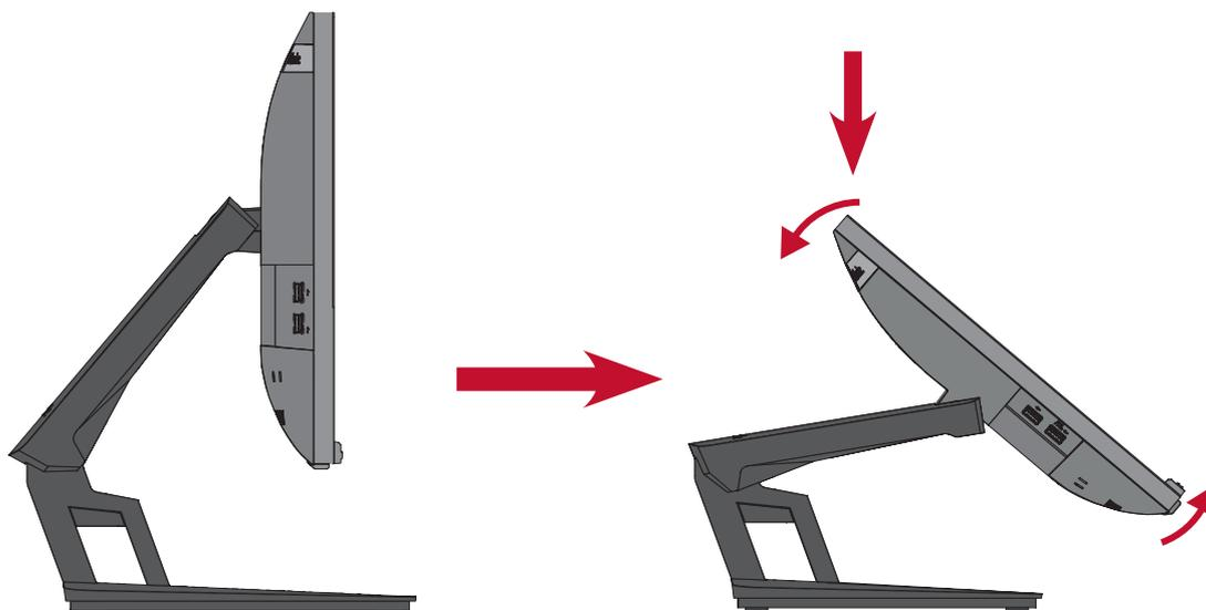
**NOTE:** When adjusting, support the stand firmly with one hand while tilting the monitor forwards or backwards with the other hand.
