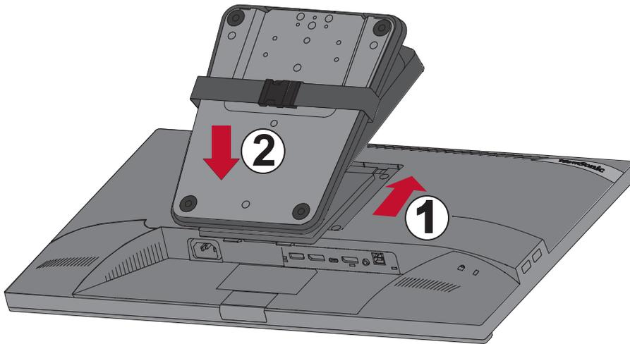
**NOTE:** Ensure the stand is secure and the quick release tab positively clicks into place.
