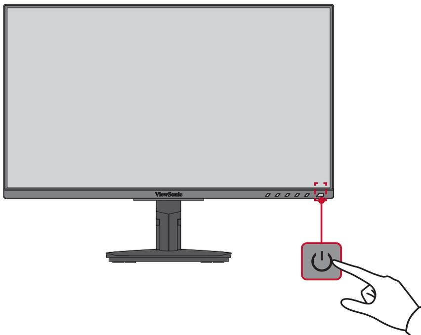
**NOTE:** The monitor will still consume some power as long as the power cord is connected to the power outlet. If the monitor is not being used for a long period of time, please disconnect the power plug from the power outlet.
