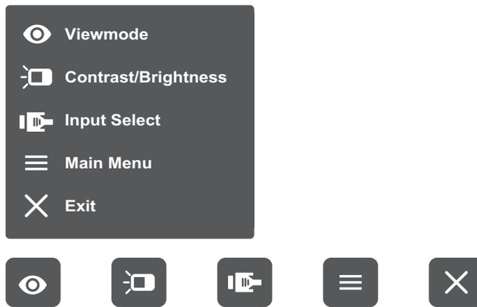
**NOTE:** Follow the key guide that appears on the bottom of the screen to select the option or make adjustments.
