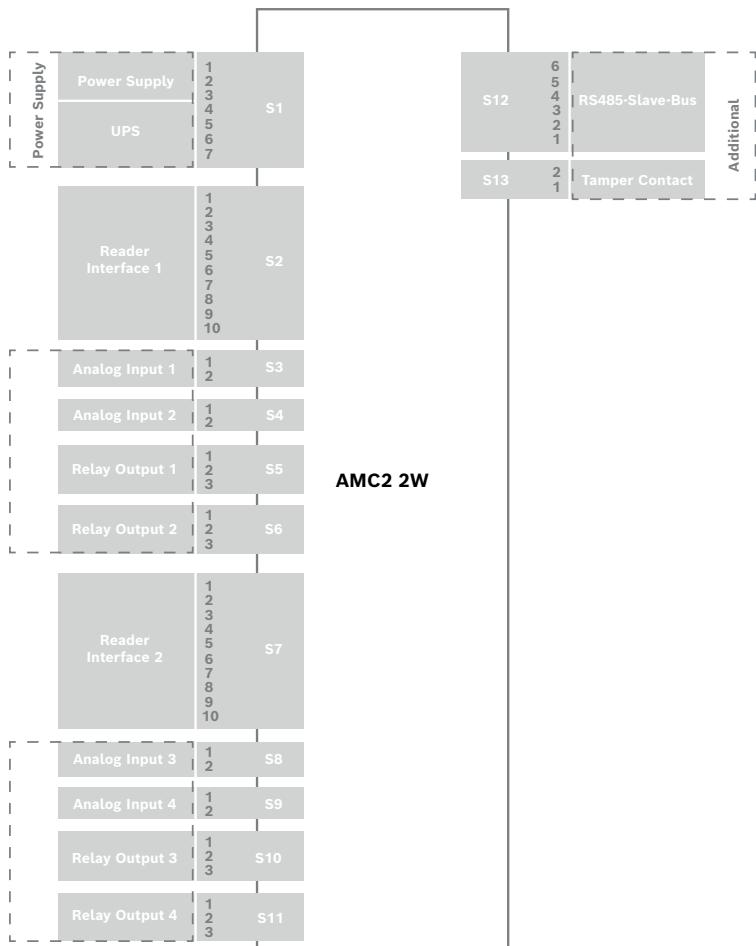
**Figure 10.3: Connector blocks of the AMC2-2W**
