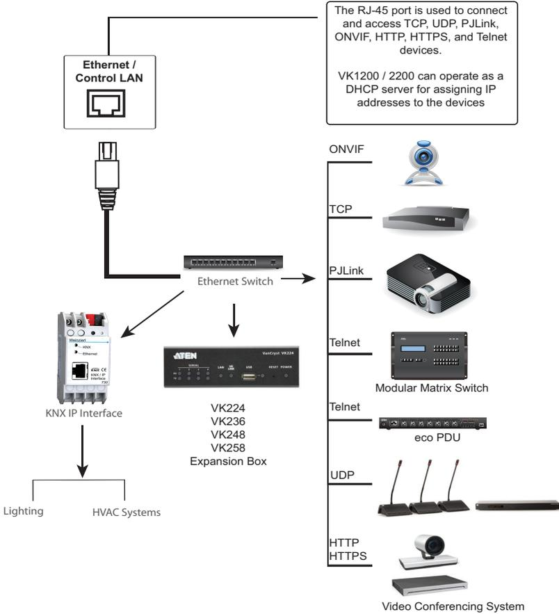
The RJ-45 port is used to connect and access TCP, UDP, PJLink, ONVIF, HTTP, HTTPS, and Telnet devices.
