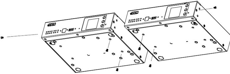
2. Use 4 of the screws from step 2 to secure the two VK1200 units together with the link bracket. Then install the left and right mounting brackets onto the sides of the units using 2 of the M3x5 and M3x6 screws included.
