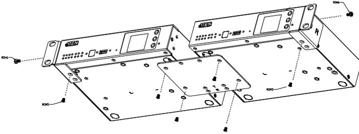
3. Align the mounting brackets' screw holes with that of the front of the rack, and secure the units onto the rack using 4 self-supplied screw.
