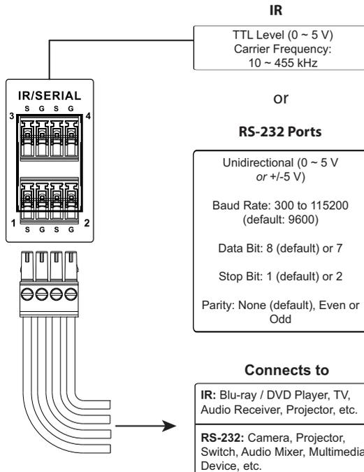
By default, the unidirectional IR / serial channels are set to transmit IR signals.
