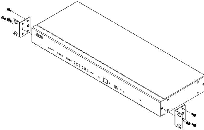
2. Align the mounting brackets' screw holes with that of the front of the rack, and use 4 self-supplied screws to secure the unit onto the rack.
