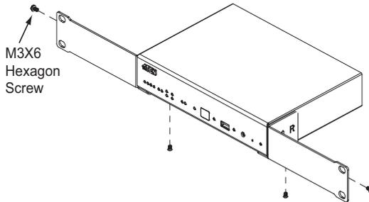
3. Use 4 self-supplied screw to secure the mounting brackets onto the rack.
