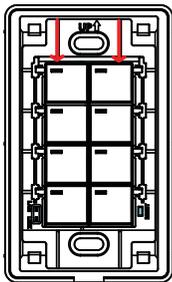
8. Mount the Control Pad to the wall.
