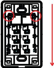
**Caution:** When removing button caps, place your fingers on the top of button caps and then press downwards, as illustrated below. Pressing upwards from the bottom may cause damages to the button caps.
