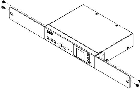
2. Align the mounting brackets' screw holes with that of the front of the rack, and secure the unit onto the rack using 2 self-supplied screws.
