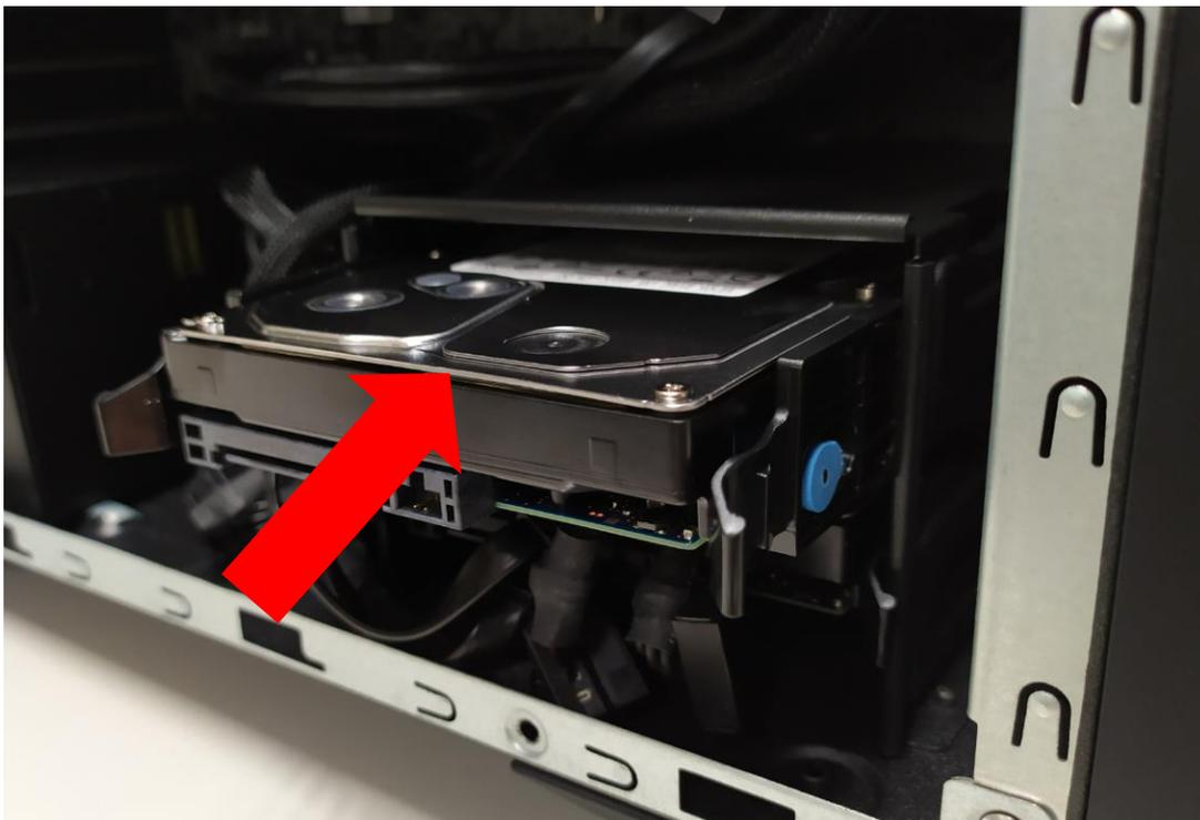
4. Connect the power and data cables to the hard drive.
