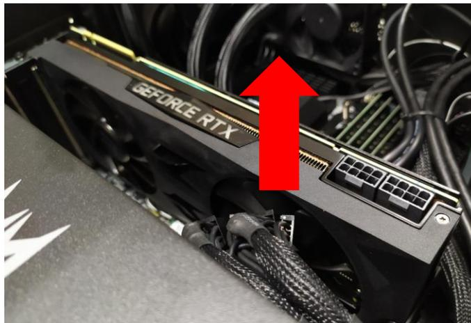
6. Remove the screw that secure the Graphic boards to the VGA Holder Bracket.
