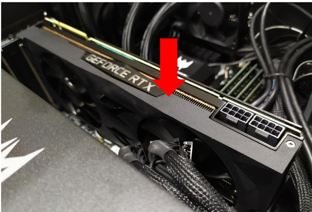
4. Secure the Graphic board with screws.
