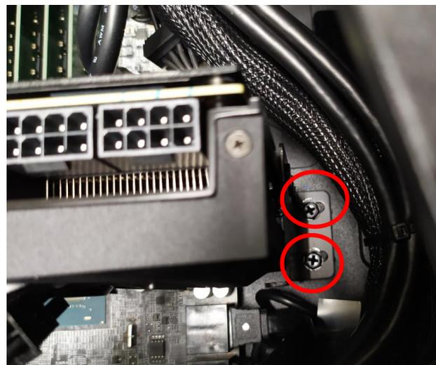
4. Release the latch that secures the graphic board to the mainboard.
