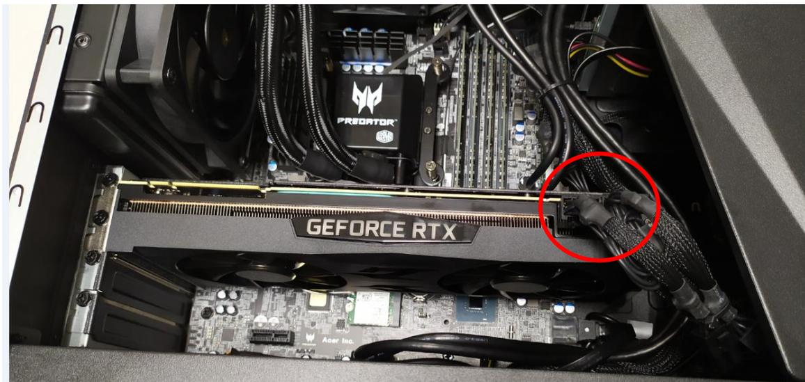
3. Remove the screw that secure the Graphic boards to the chassis.
