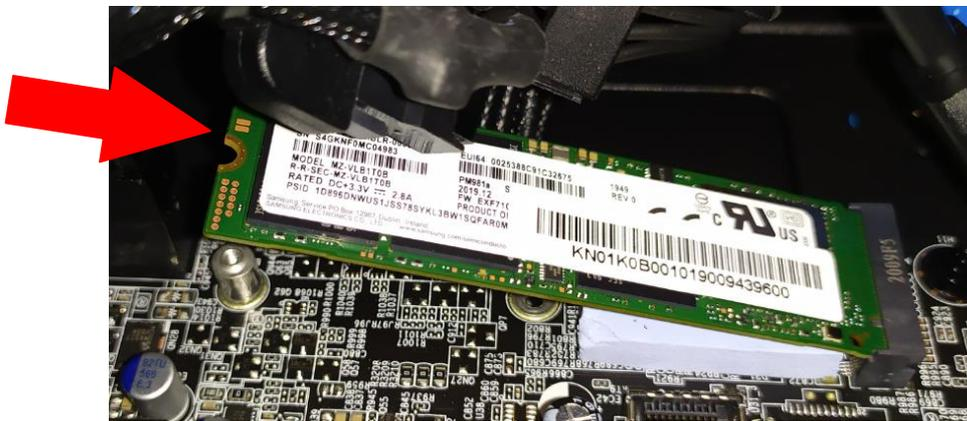
3. Secure the M.2 SSD module and mainboard with screws.
