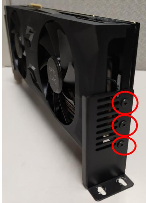
3. Insert the Graphic boards into the PCIe x16 slot and press it down until it latches into place.
