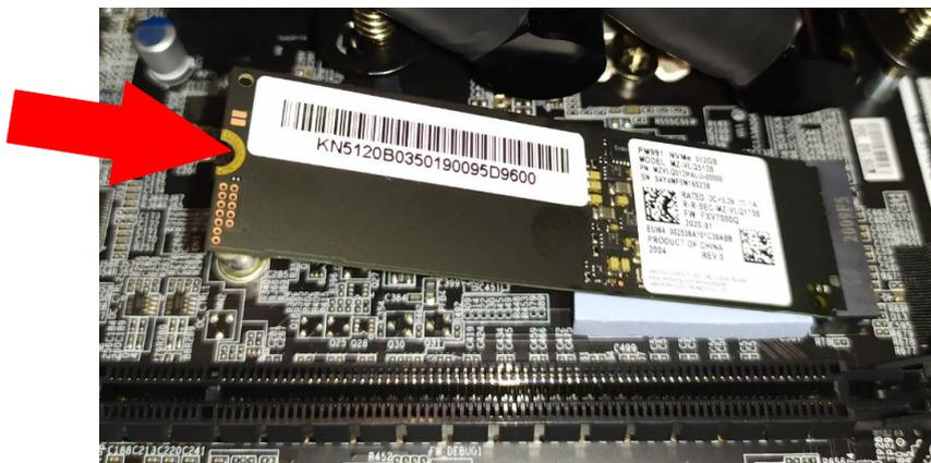
3. Secure the M.2 SSD module and mainboard with screws.
