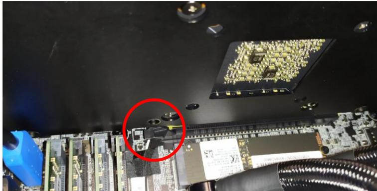
5. Detach the Graphic board from the PCIe x16 slot.
