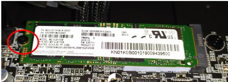
4. Detach the M.2 SSD module from the mainboard.
