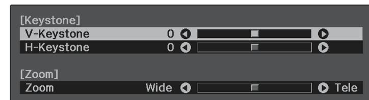
**3** Use the arrow buttons on the remote control to select between vertical and horizontal keystone correction and to adjust the image shape as necessary.
