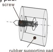
3. Make screw in alignment with the hole on lower base cover. Fasten rubber supporting pad to the base cover firmly by a cross screw driver (self-provided).
