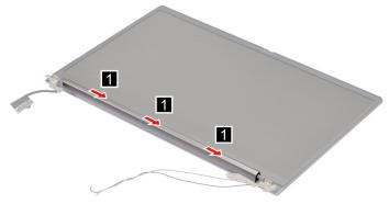
Figure 89. Remove the hinge cover
