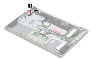
Figure 29. Remove the fingerprint board with cable
