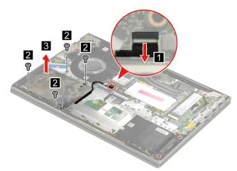
Figure 56. Remove four screws and then remove the HDD module
