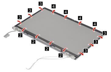
Figure 91. Remove the LCD bezel
