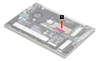
Figure 19. Remove the memory module shielding
