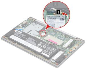
Figure 34. Peel off the mylar
