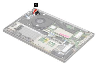
Figure 70. Peel off the tape
