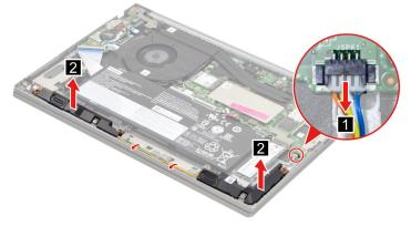
Figure 74. Remove the speakers
