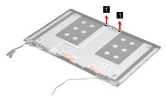
Figure 44. Remove the microphone rubbers
