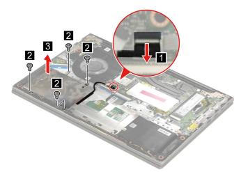
Figure 14. Remove four screws and then remove the HDD module
