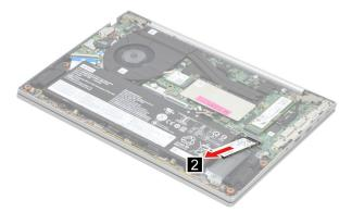
Figure 12. Remove the 2<sup>nd</sup> SSD by pulling it away from the slot
