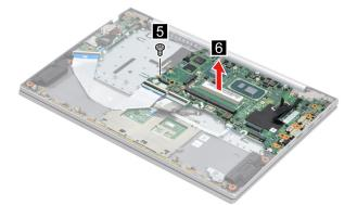
Figure 33. Remove one screw and then remove the system board
