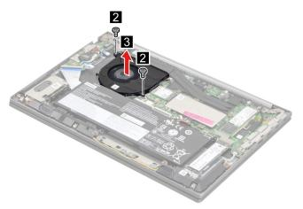
Figure 61. Remove two screws and then remove the fan
