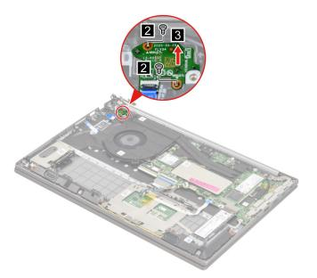
Figure 71. Remove two screws and remove the power board with cable
