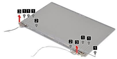
Figure 92. Remove eight screws and remove the hinges
