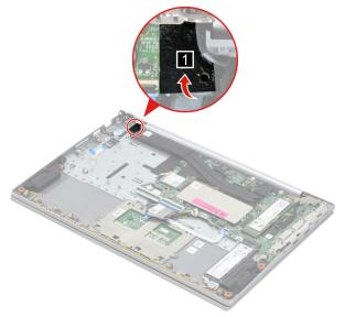
Figure 27. Peel off the tape
