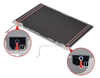
Figure 41. Remove the two pieces of removable tape with tweezers
