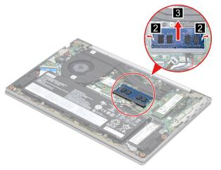
Figure 20. Remove the memory module
