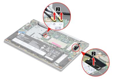
Figure 35. Detach the antenna cable connectors and disconnect the EDP cable form the system board
