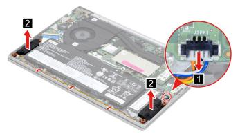
Figure 31. Remove the speakers
