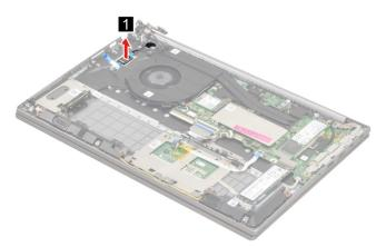
Figure 72. Remove the fingerprint board with cable
