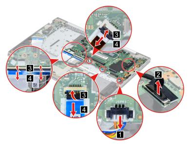
Figure 32. Disconnect cables connected to the system board
