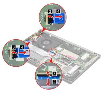
Figure 68. Disconnect the I/O board cable from the system board and disconnect the fingerprint board cable and the power board cable from the I/O board
