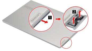
Figure 46. Eject the earphone tray and then remove the Bluetooth headset
