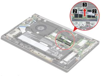
Figure 63. Remove the memory module
