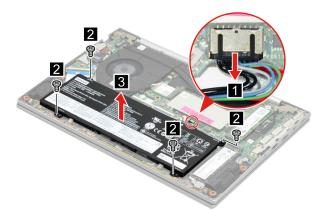
Figure 7. Remove four screws and remove the battery pack
