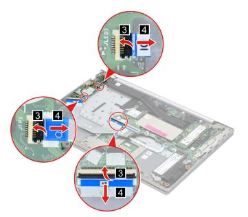
Figure 25. Disconnect the I/O board cable from the system board and disconnect the fingerprint board cable and the power board cable from the I/O board
