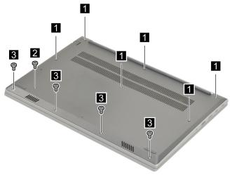
Figure 47. Loosen six screws and remove five screws
