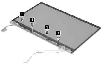
Figure 90. Remove three screws
