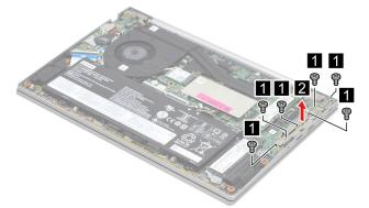
Figure 22. Remove six screws and then remove the I/O bracket (left)
