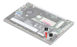
Figure 13. Remove one screw and remove the 2<sup>nd</sup> SSD bracket
