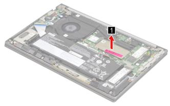
Figure 62. Remove the memory module shielding
