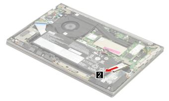
Figure 54. Remove the 2<sup>nd</sup> SSD by pulling it away from the slot
