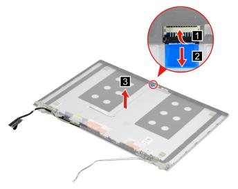
Figure 43. Disconnect the EDP cable from the camera board and remove the EDP cable
