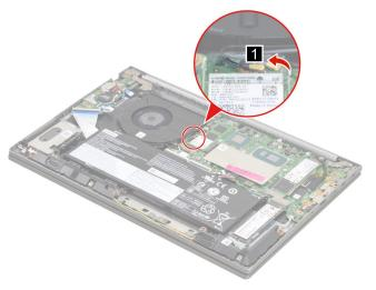
Figure 86. Peel off the mylar
