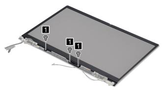
Figure 38. Remove three screws
