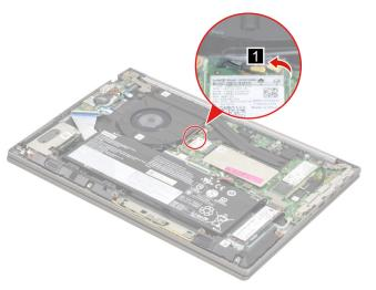
Figure 57. Peel off the mylar
