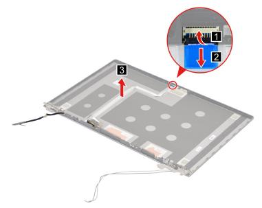
Figure 95. Disconnect the EDP cable from the camera board and remove the EDP cable
