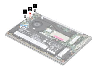
Figure 23. Remove two screws and remove the I/O bracket (right)
