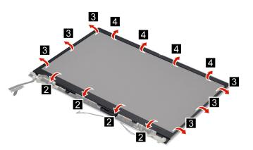
Figure 39. Remove the LCD bezel
