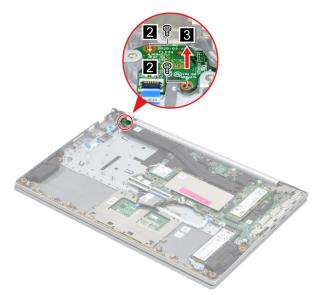
Figure 28. Remove two screws and remove the power board with cable
