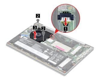
Figure 18. Remove two screws and remove the fan
