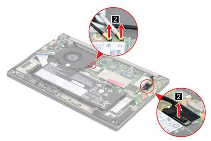
Figure 87. Detach the antenna cable connectors and disconnect the EDP cable form the system board
