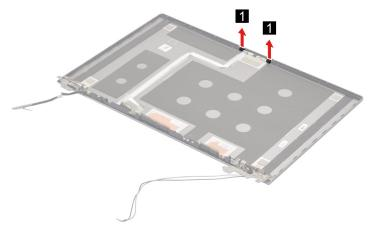
Figure 96. Remove the microphone rubbers
