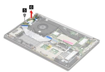
Figure 69. Remove one screw and remove the I/O board with cable
