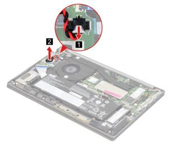
Figure 64. Disconnect the CMOS battery cable from the I/O board and remove the CMOS battery
