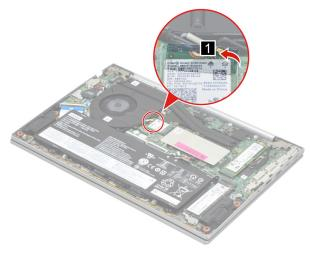
Figure 15. Peel off the mylar
