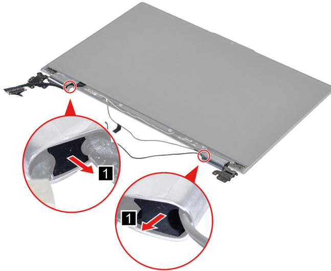
Figure 33. Remove the rubber hinges
