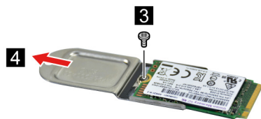
Figure 9. Remove one screw and separate the SSD from the SSD bracket
