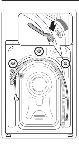
1. Locate the shipping bolts (marked with circle in the figure) on the rear side of the washing machine.
