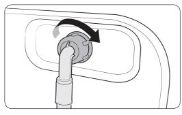
1. Connect the water hose to the water tap, and then turn it to the right to tighten.
