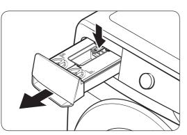
1. While holding down the **release lever** on the inner of the drawer, pull the detergent drawer to remove.
