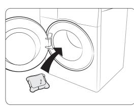
1. Put the capsule in the bottom of the empty drum towards the rear.
