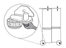
1 Open the door and use the spanner ① to loosen the keeper nut by turning it to the left.
