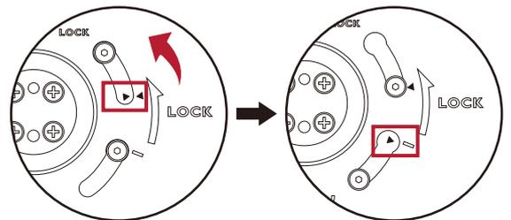
Raise the thumbscrew lids and tighten the thumbscrews as illustrated. Then push the lids back.
