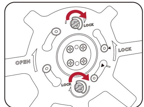
Orient and align the stand arm with the monitor, then push them together until they click and lock into place.
