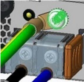
**NOTE:** To uninstall the cable from the 1300W DC PSU, remove the plastic cover and unscrew the M4 and M5 screws. Pull the 1300W DC cable out from the 1300W DC PSU socket.
