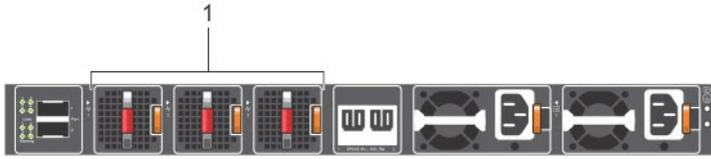
1. Fans—Fan1 is near the left edge of the switch; Fan3 is near the center of the switch.
