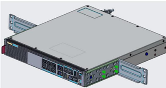
3. Attach the standard brackets to the switch using four screws for each bracket.
