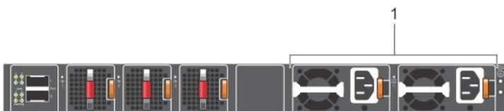
1. Default PSU and ordered-separately PSU. PSU1 is near the center of the switch; PSU2 is on the right edge of the switch.
