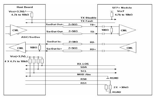
**Recommended High-speed Interface Circuit**
