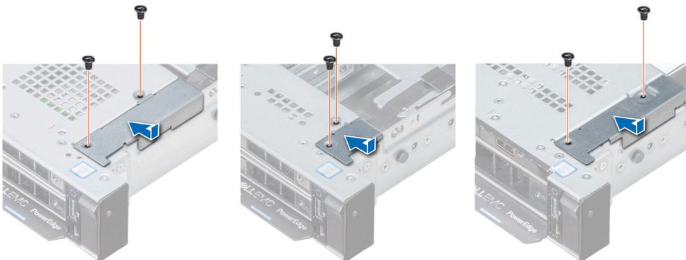
Figure 120. Installing the cable cover
