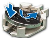
**Figure 99. Installing the system battery**
