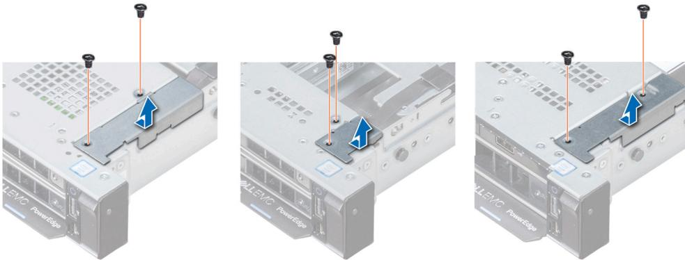
Figure 117. Removing the cable cover
