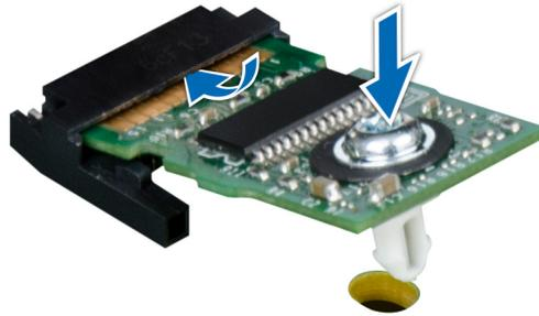
Figure 112. Installing the TPM
