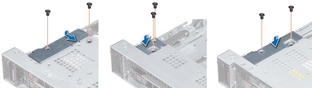
**Figure 116. Installing the cable cover**
