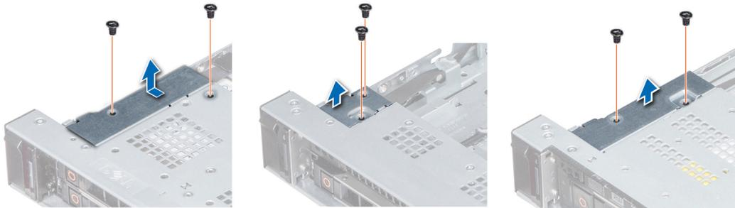
Figure 113. Removing the cable cover
