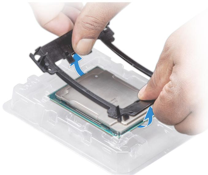
**Figure 46. Removing the processor bracket**
