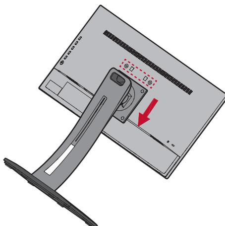
5. Attach the mounting bracket to the VESA mounting holes at the rear of the monitor. Then secure it with four (4) screws (M4 x 10 mm).
