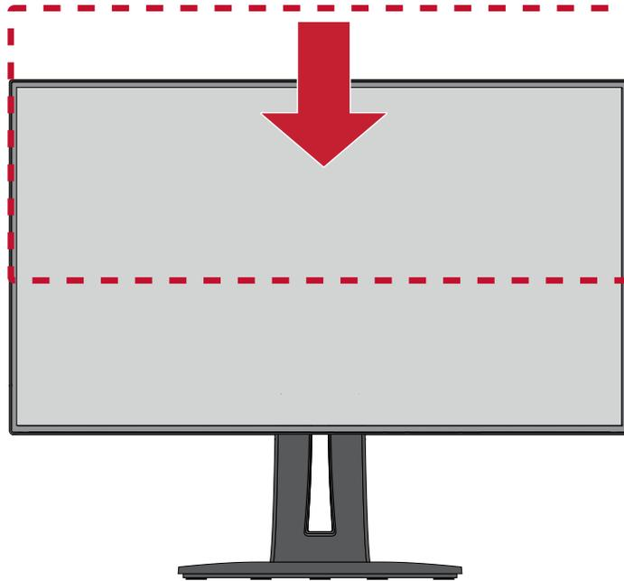
**NOTE:** When adjusting, press down firmly along the adjustment track holding the monitor with both hands on the side.
