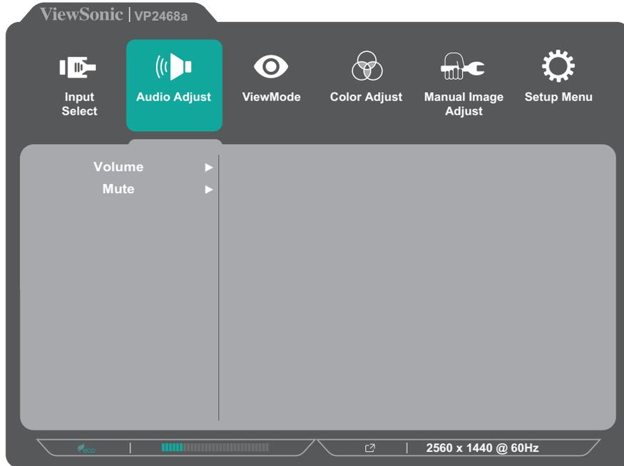
3. Press the **1** or **2** key to select the desired option. Then press the **3** key to enter its sub-menu.
