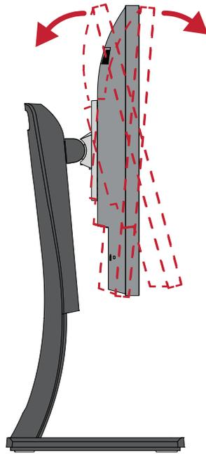
**NOTE:** When adjusting, support the stand firmly with one hand while tilting the monitor forwards or backwards with the other hand.
