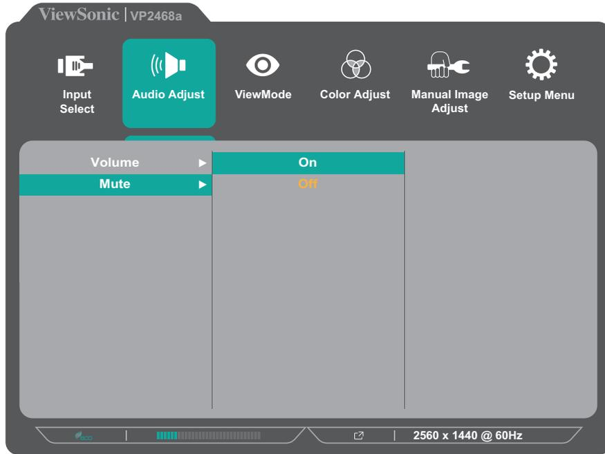
4. Press the **1** or **2** key to adjust/select the setting. Then press the **3** key to confirm.
