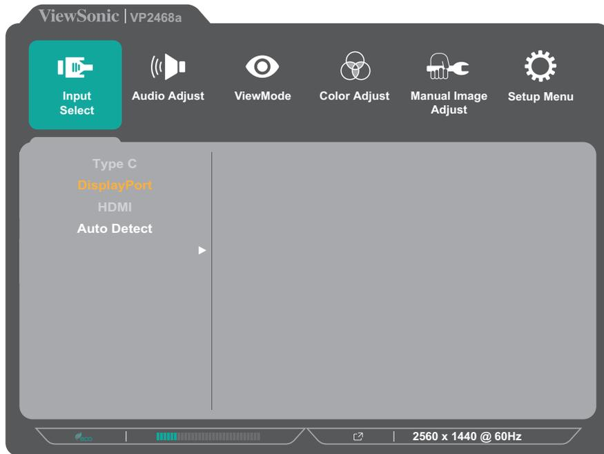
3. Press the **1** or **2** key to select the desired input source. Then press the **3** key to confirm the selection.
