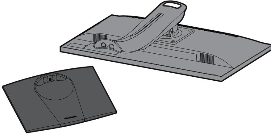
2. Align and connect the two (2) points on the monitor stand's base with the monitor stand's neck.
