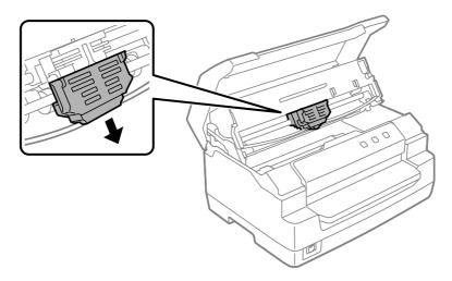
7. Hold both sides of the ribbon cartridge with both hands and rotate it on the plastic hooks. Then pull it up until it is out of the printer.
