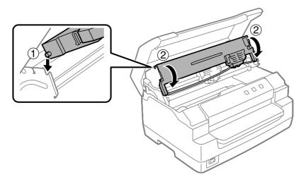
10. Hold both sides of the ribbon guide and pull it down until it is out of the cartridge.
