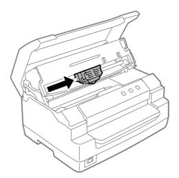
6. Hold both sides of the ribbon guide and pull it down until it is out of the print head.
