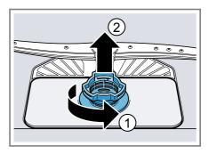
Pull down the micro filter to remove.
