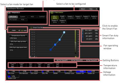
• Smart Fan - This setting enables/disables the Smart Fan function. Smart Fan is an excellent feature which will adjust the CPU/system fan speed automatically depending on the current CPU/system temperature, avoiding the overheating to damage your system.
