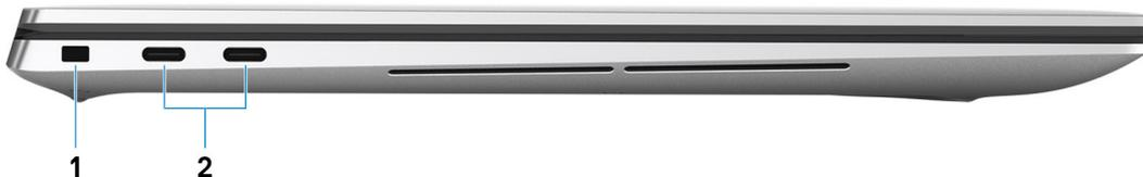
**1. Security-cable slot (wedge-shaped)**
