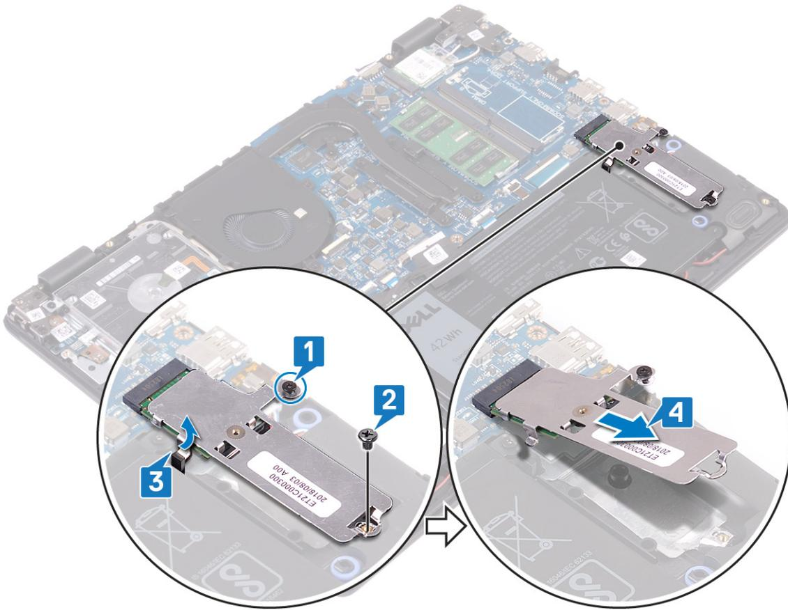
5. Turn the solid-state drive shield/Intel Optane shield over.
