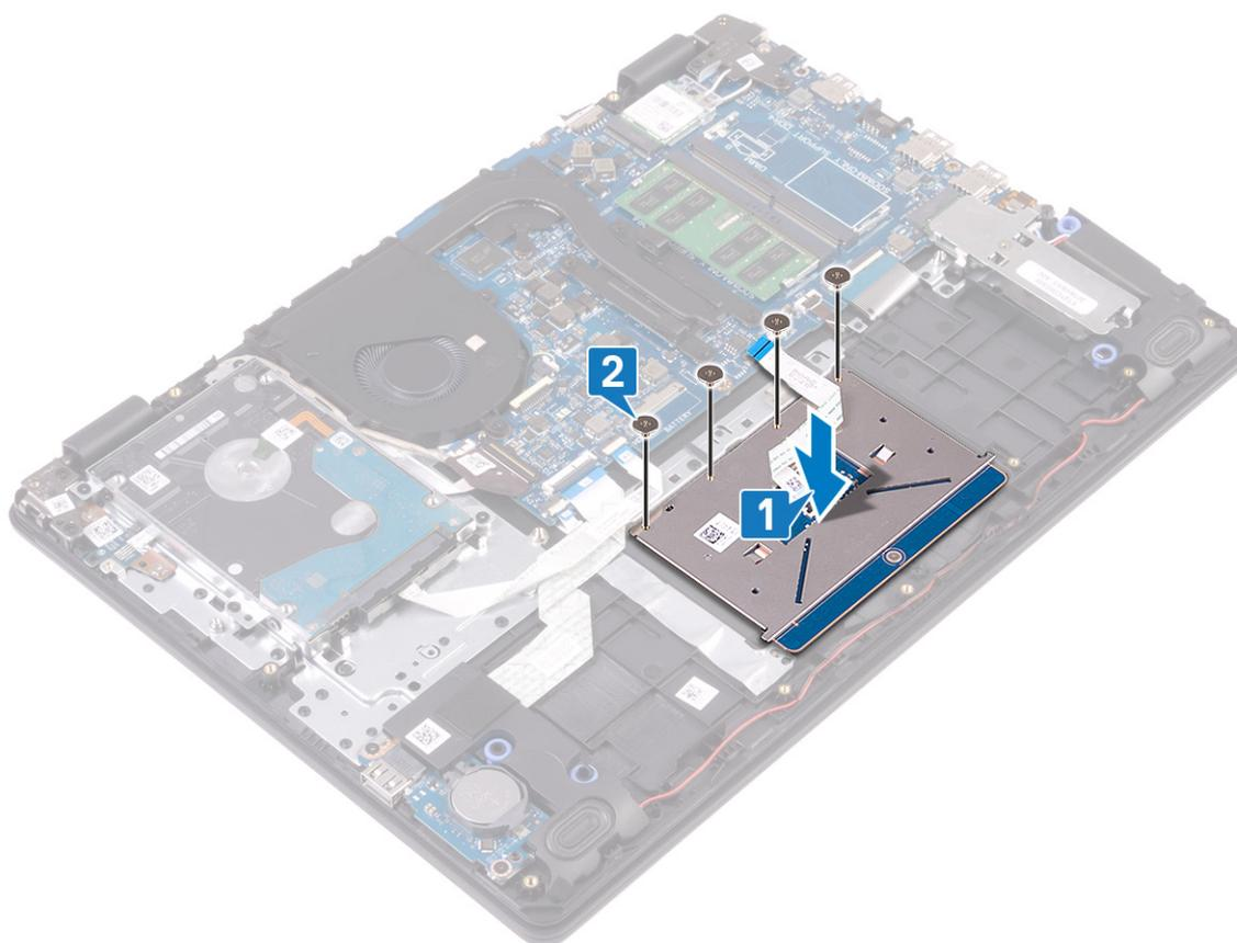
3. Place the touchpad bracket into the slot on the palm rest and keyboard assembly.
