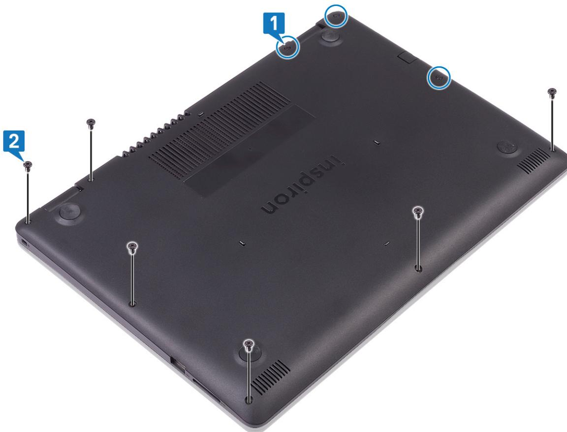
3. Pry the base cover from the top-right corner of the palm-rest and keyboard assembly.
