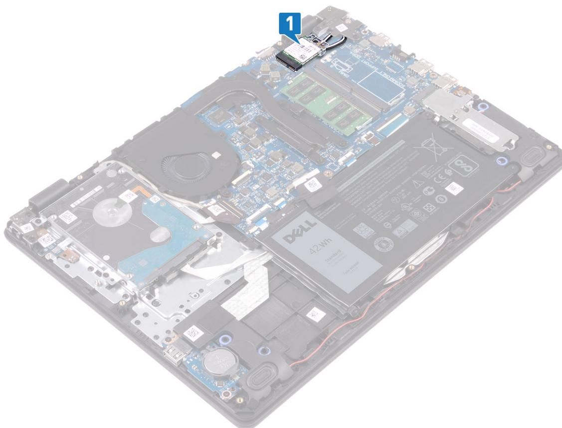
2. Remove the screw (M2x3) that secures the wireless-card bracket to the system board.
