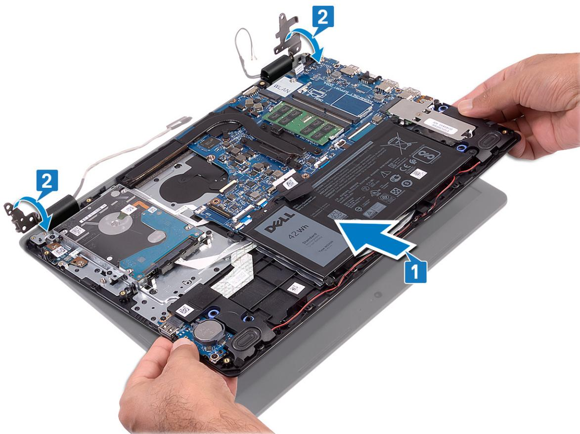
3. Replace the four screws (M2.5x4) that secure the display hinges to the system board and I/O board.
