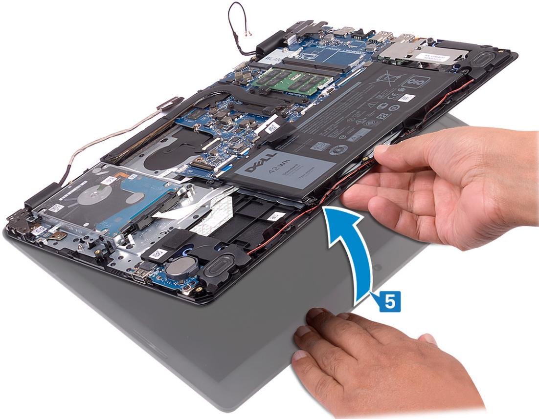
6. Slide and remove the palm-rest and keyboard assembly off the display assembly.
