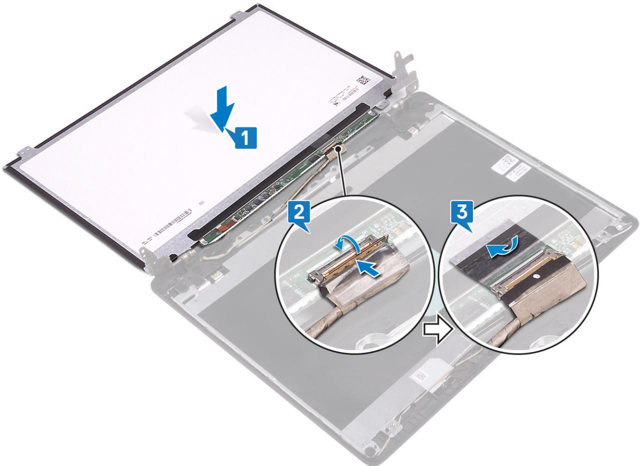
4. Turn the display panel over and place it on the display back-cover and antenna assembly.
