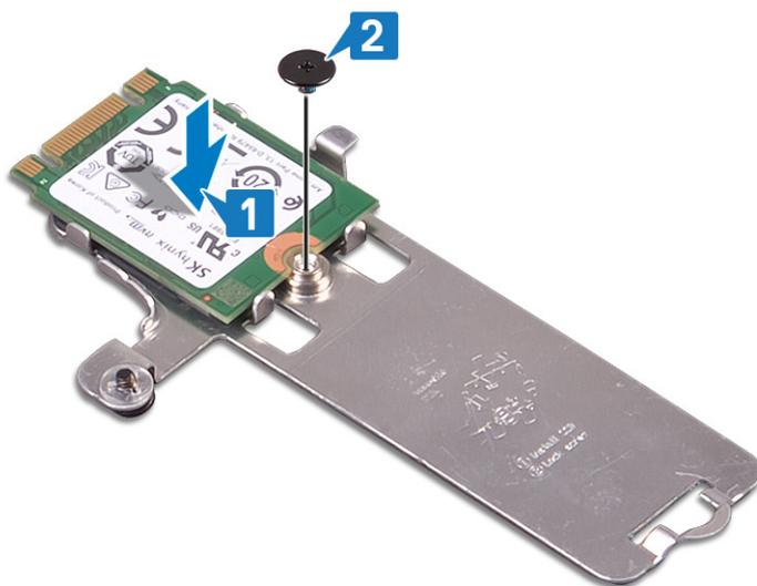
3. Align the notch on the solid-state drive/Intel Optane with the tab on the solid-state drive/Intel Optane slot.
