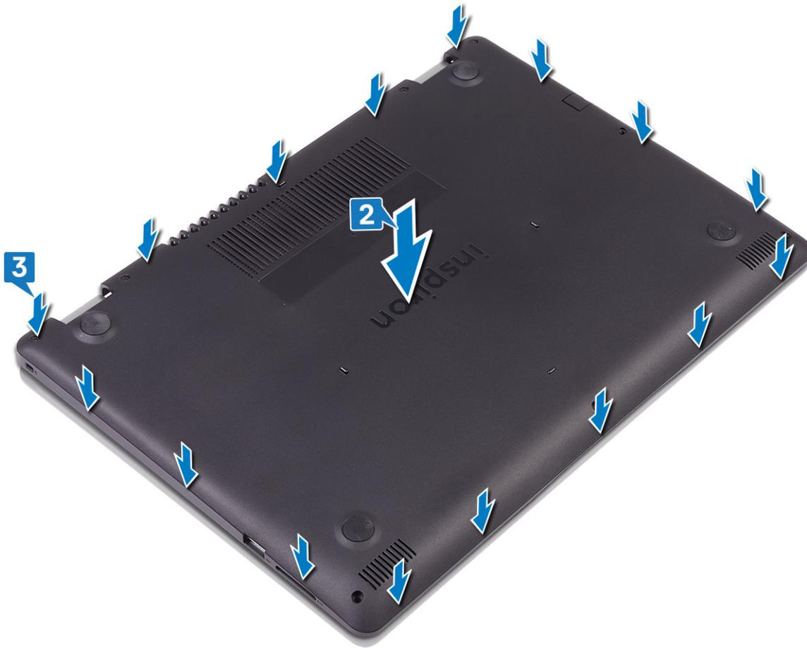
4. Replace the six screws (M2.5x4) that secure the base cover to the palm-rest and keyboard assembly.
