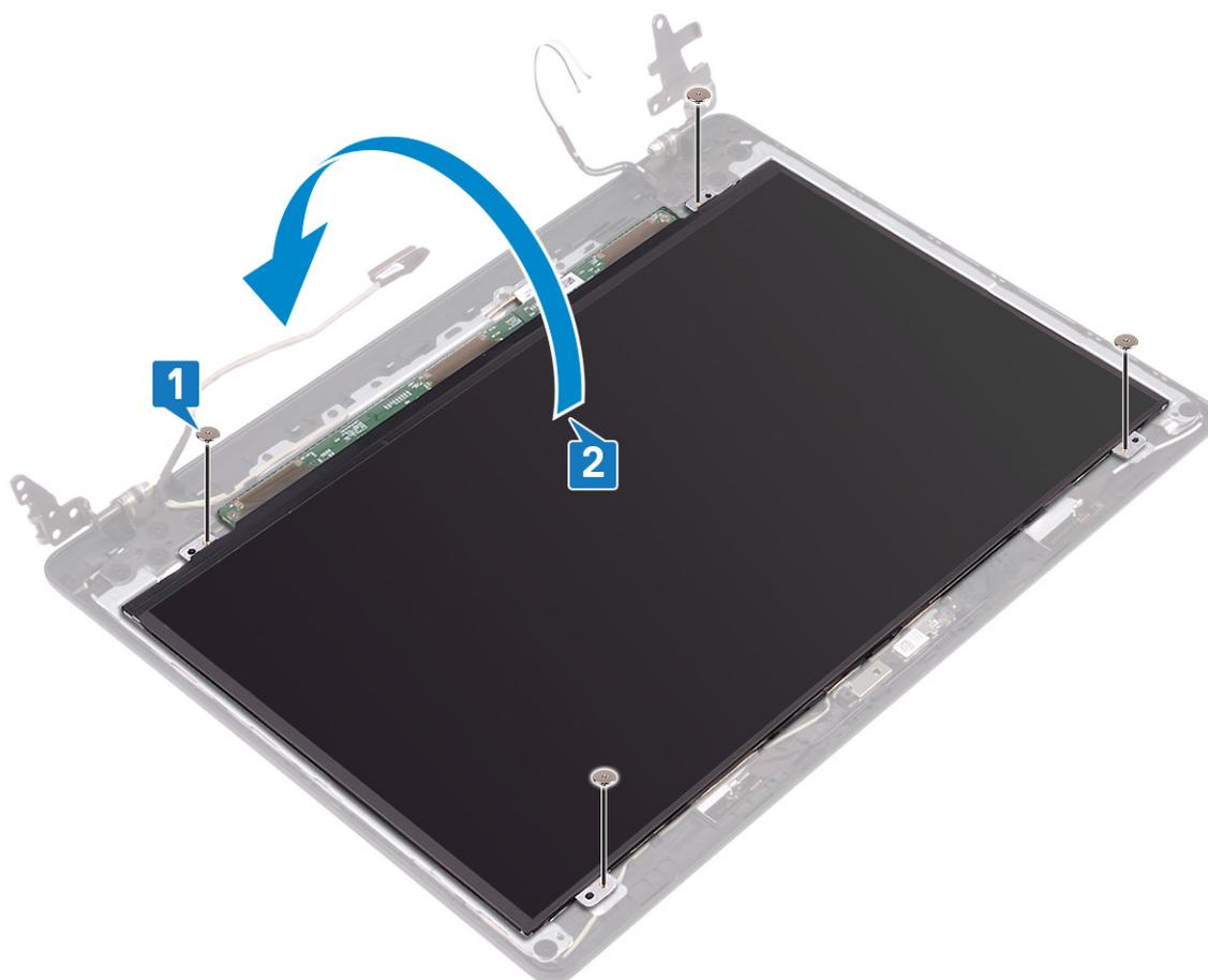
3. Peel the tape that secures the display cable to the back of the display panel.
