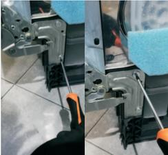
6. Remove the hinge screws
