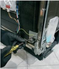
8. Remove the front hinge screw
