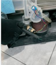
4. Remove the hinge spring
