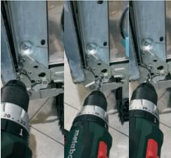
5. Drill the hinge rivets
