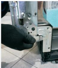
10. Fit the new hinge with riveter
