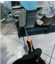
11. Fix the lateral hinge screws
