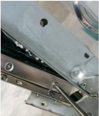
9. Remove the lateral hinge screws
