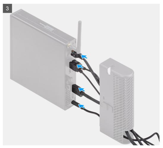
$\textbf{7.} \ \ \text{Align the cable cover retaining hooks into the slots on the OptiPlex 5080 Micro chassis.}$
