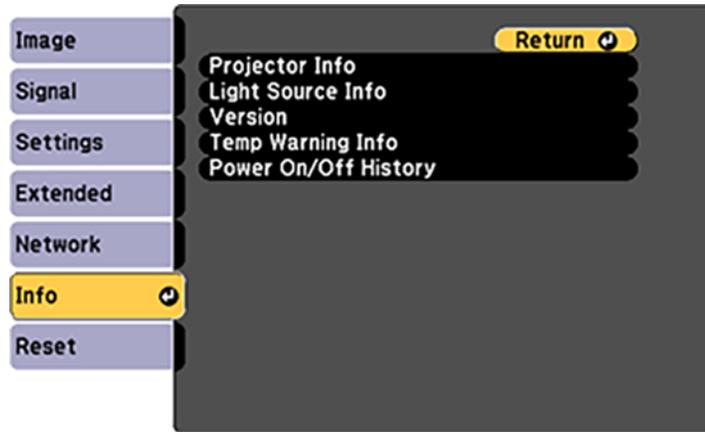
Select **Light Source Info** to display the projector's light source information. Select **Version** to display the projector's firmware version. Select **Temp Warning Info** to display the projector's high temperature warnings. Select **Power On/Off History** to display the projector's power on and off history. Select **Projector Info** to display the settings described below.
