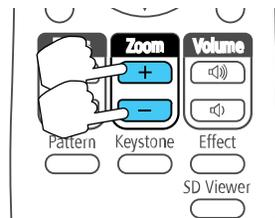
**Note:** When minimizing the size of the image using the optical zoom, a message is displayed and the projector switches to digital zoom. When maximizing the size of the image using the digital zoom, a message is displayed and the projector switches to optical zoom.
