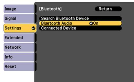
6. Turn on pairing mode on the Bluetooth audio device you want to connect to. (See your Bluetooth audio device manual for details.)
