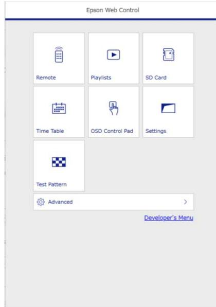
4. To control projection remotely, select the **Remote** option from the Epson Web Control screen.
