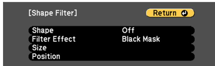
4. To change the shape of the effect, select **Shape**, press **↵ Enter**, select a shape option, and press **Menu** to exit.
