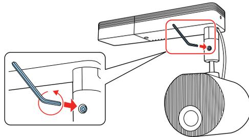
**Warning:** Do not grip the ball joint with your fingers while loosening the screw or your fingers could get pinched.
