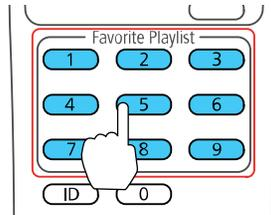
**Note:** You can assign playlists to each of the number buttons (1 to 9) on the projector's remote control using the Epson Projector Content Manager software. See the *Epson Projector Content Manager Operation Guide* for details.
