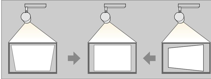
**Note:** You cannot combine **Keystone** correction with other image shape correction methods. You can correct horizontal keystone distortion up to 40° right or left, and vertical keystone distortion up to 45° up or down.
