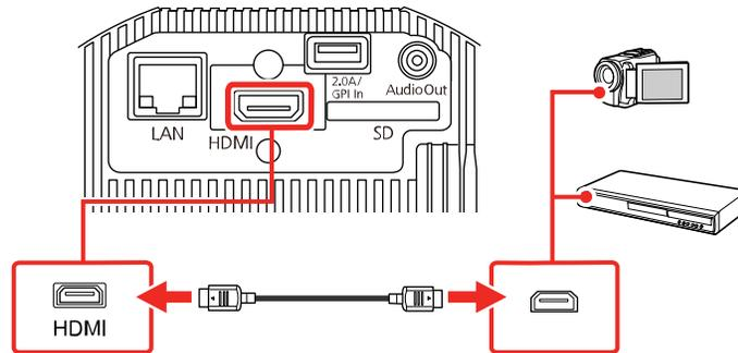
**Note:** The projector converts the digital audio signal sent from your video source into a stereo analog signal if you are connecting to external speakers.
