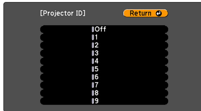
5. Press the arrow buttons on the remote control to select the identification number you want to use for the projector. Then press **↵ Enter**.
