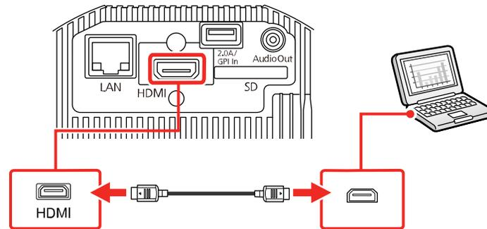
**Note:** The projector converts the digital audio signal sent from your computer into a stereo analog signal if you are connecting to external speakers. (Make sure the HDMI audio playback device on your computer's audio settings is set to **EPSON PJ.**)
