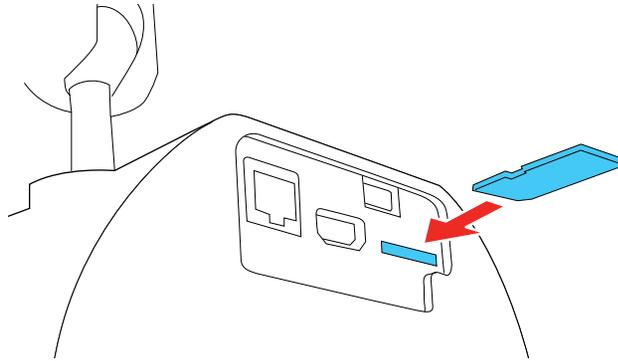
**Note:** Insert the SD card directly into the projector. Do not use a hub or your settings may not be saved correctly.
