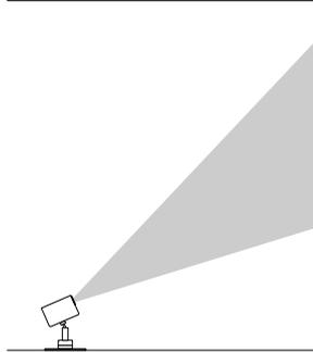
**Note:** Use the direct mount (included) only for mounting the projector on a wall or ceiling. If installing on a lighting track, use only the optional lighting track mount (ELPMB66). If you do not mount the projector, use only the optional floor stand (ELPMB55).
