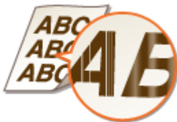
Streaks Appear/Printing is Uneven
