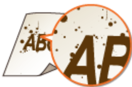
Toner smudges and splatters appear
