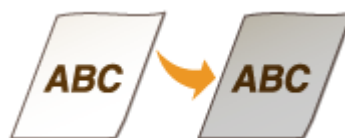
Blank space of originals becomes grayish in printouts
