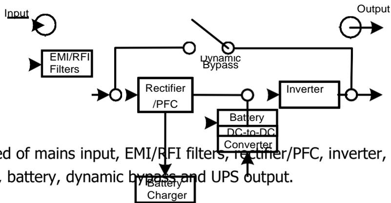
The UPS is composed of mains input, EMI/RFI filters, rectifier/PFC, inverter, battery charger, DC-to-DC converter, battery, dynamic bypass and UPS output.
