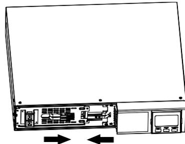
Re-connect the battery wires.
