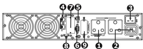
1. Programmable outlets: connect to non-critical loads.
