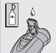
**3** Lubricate the trimmer teeth with a drop of sewing machine oil every six months.
