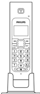
7. Please note that handset may not turn ON for up to 15 minutes if the batteries are too low. Before first use, put the product on the charger and charge batteries for 24 hours minimum. The handset may get warm during the initial charge. This is normal.
