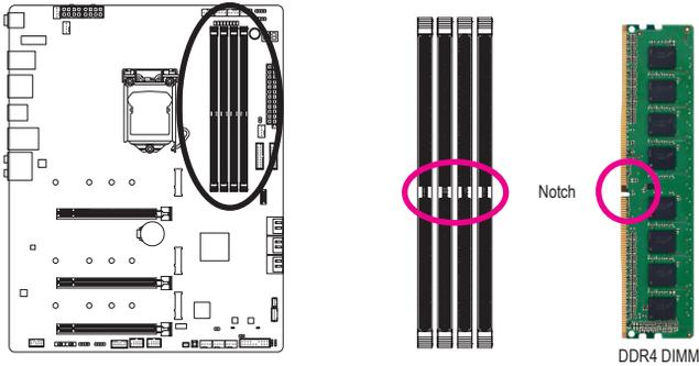
A DDR4 memory module has a notch, so it can only fit in one direction. Follow the steps below to correctly install your memory modules in the memory sockets.
