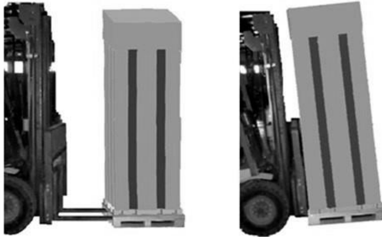
Figure 2-2 Moving the Equipment using a Forklift Truck
