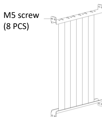
Figure 3-24 Fixed Mode of the Supply Air Baffle
