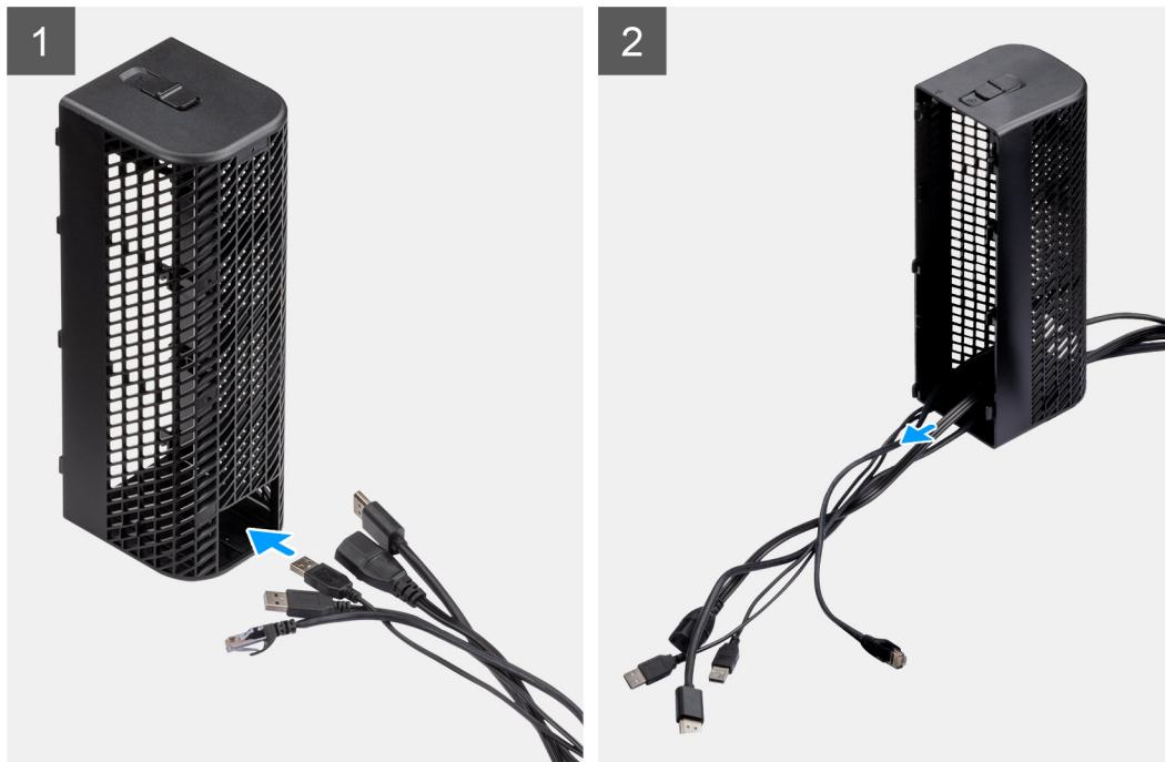
3. Connect the cables to their respective ports and turn the antenna (if available/applicable) outwards to pass through the antenna slot at the top of the cable cover.
