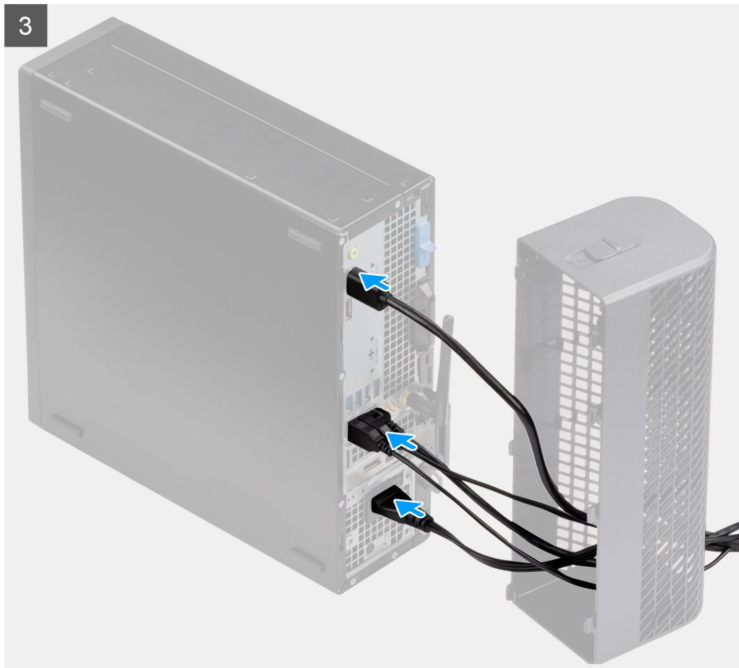
4. Align the cable cover retaining hooks into their slots on the Dell OptiPlex Small Form Factor chassis.
